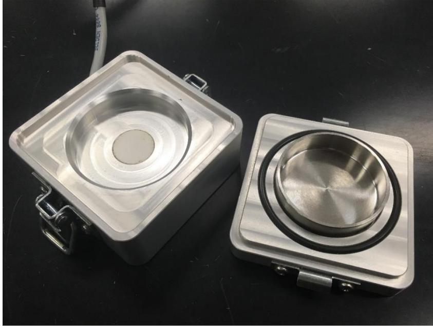
Figure D.3 Water activity meter for measuring  $a_w$  at high temperature.
