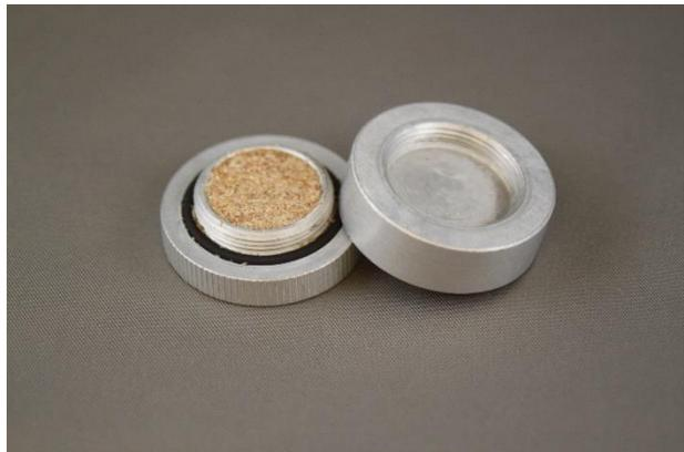
Figure D.4 Example of almond products in plastic bag and aluminum test-cell for thermal inactivation studies.
