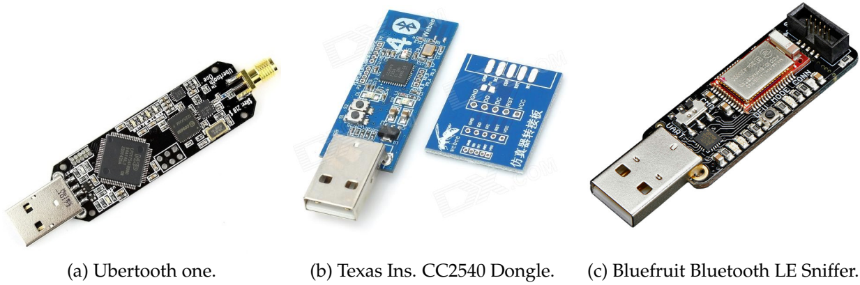
Figure 3.1: Narrowband sniffers utilize Bluetooth-compliant radios to capture Bluetooth packets. This figure presents three samples including (a) Ubertooth one, (b) Texas Instrument CC2540 USB Dongle Bluetooth LE sniffer, and (c) Bluefruit Bluetooth LE sniffer.
