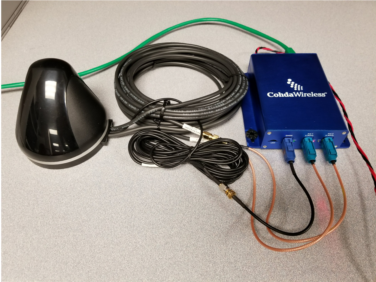
Figure 6.3 Setup of measurements using two MK5 units over a stationary link. The antenna is MGW-303 which includes two WiFi antennas and a GPS antenna.
