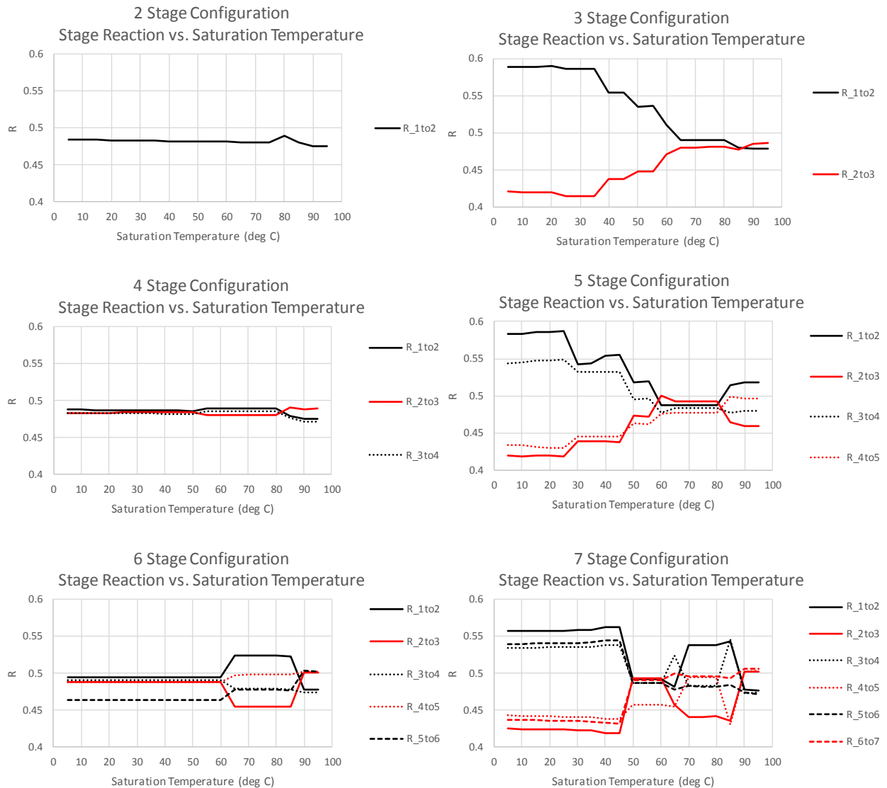
Figure 6.40. Counter-Rotating Reaction Pairs vs. Saturation Temperature at First Rotor Inlet
