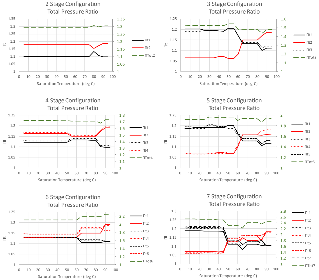
Figure 6.45. Total Pressure Ratio vs. Saturation Temperature at First Rotor Inlet
