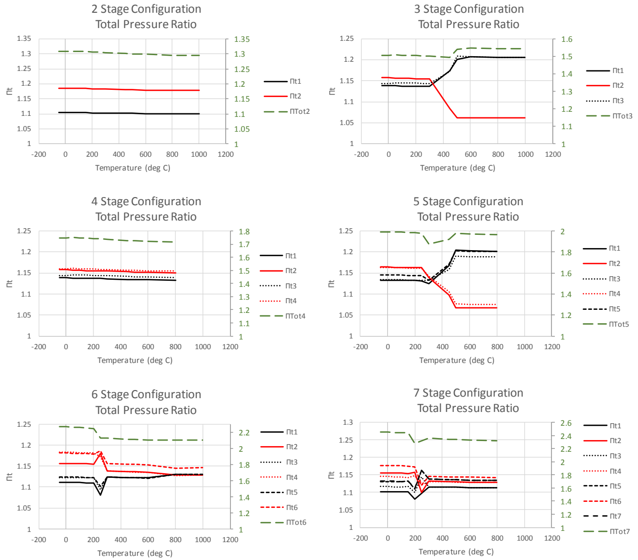
Figure A6.1.12 Total Pressure Ratio vs. Temperature at First Rotor Inlet (Air)
