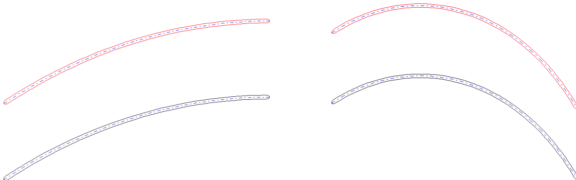
Figure 5.7. Blade-to-Blade View at Hub of Left: 90°-Limited Case, Right: Full Free-Vortex Turning
