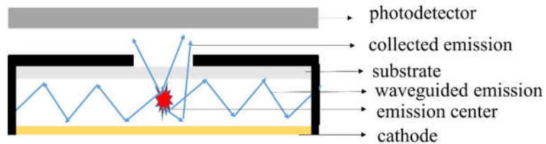
Figure 3.16 Forward emitted vs edge emitted light from the OLED device.
