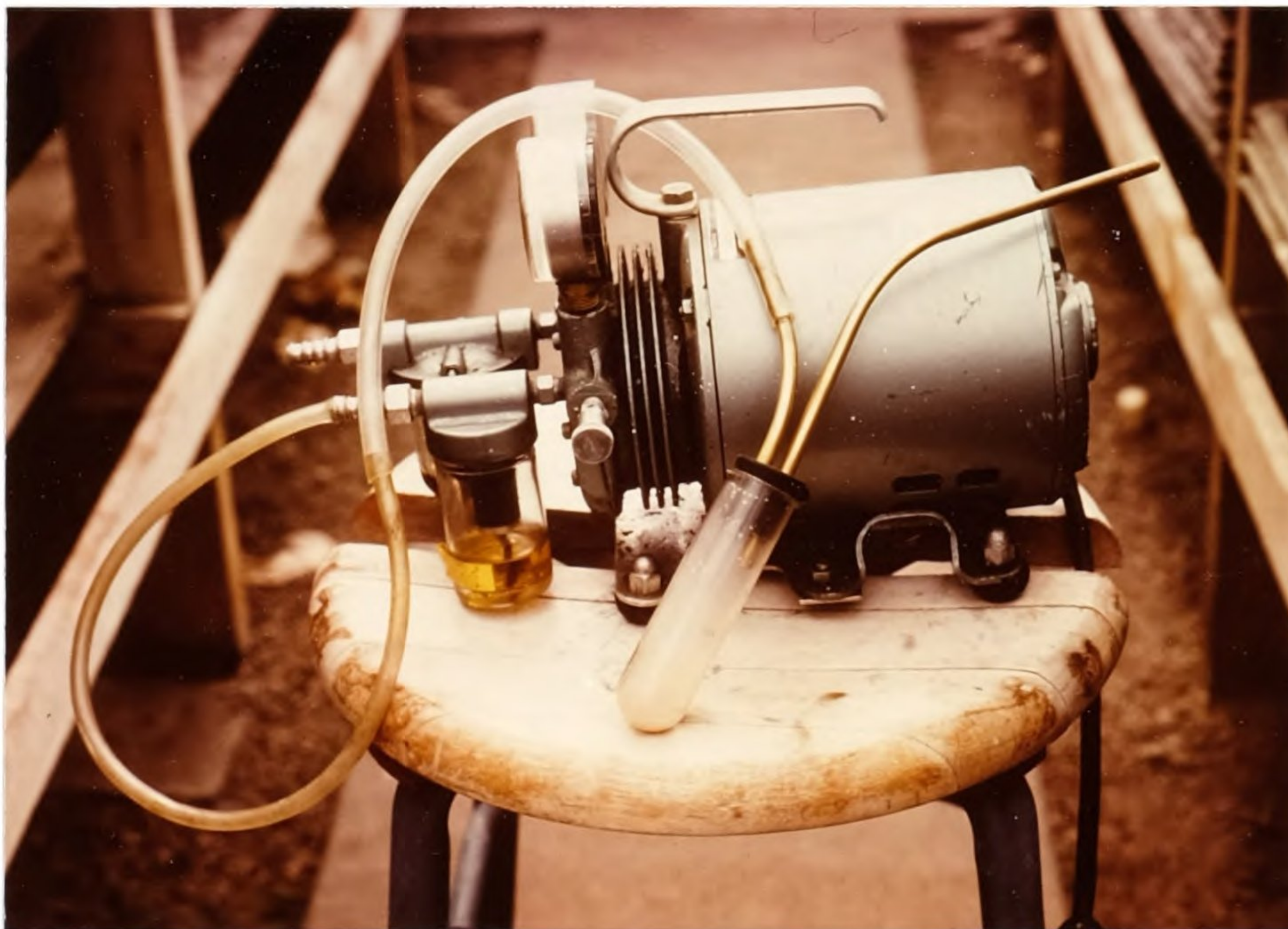
Figure 3. Aspirator apparatus used to collect whitefly adults.
