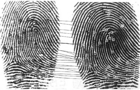
Figure 1.11: Example of fingerprint matching. Two impressions of the same finger from FVC 2002 DB1 [26] with 37 and 38 minutiae, respectively. 25 true correspondences are found here.
