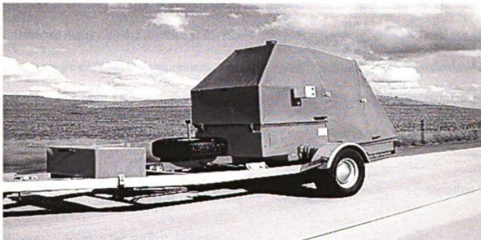
Figure 2.9 KUAB falling weight deflectometer
