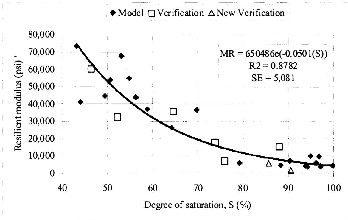
Figure 4.4 MR versus the degree of saturation (S, see table 4.1) for the SC, CL and ML soils
