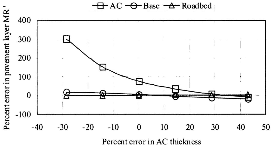
Figure 4.7 Effect of AC layer thickness on MR
