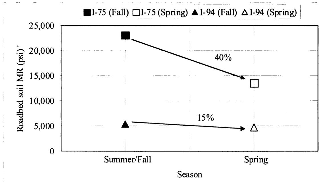
Figure 4.30 Partial spring condition FWD testing
