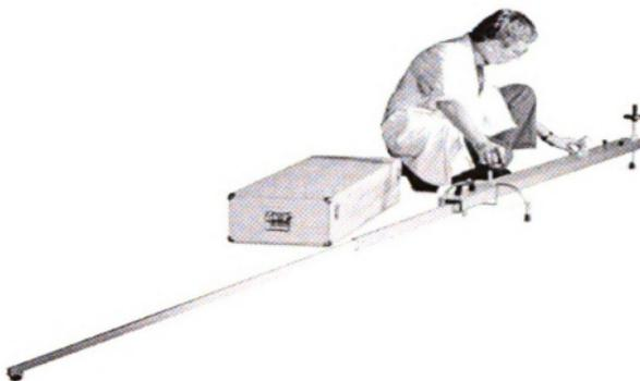
Figure 2.4 Benkelman beam
