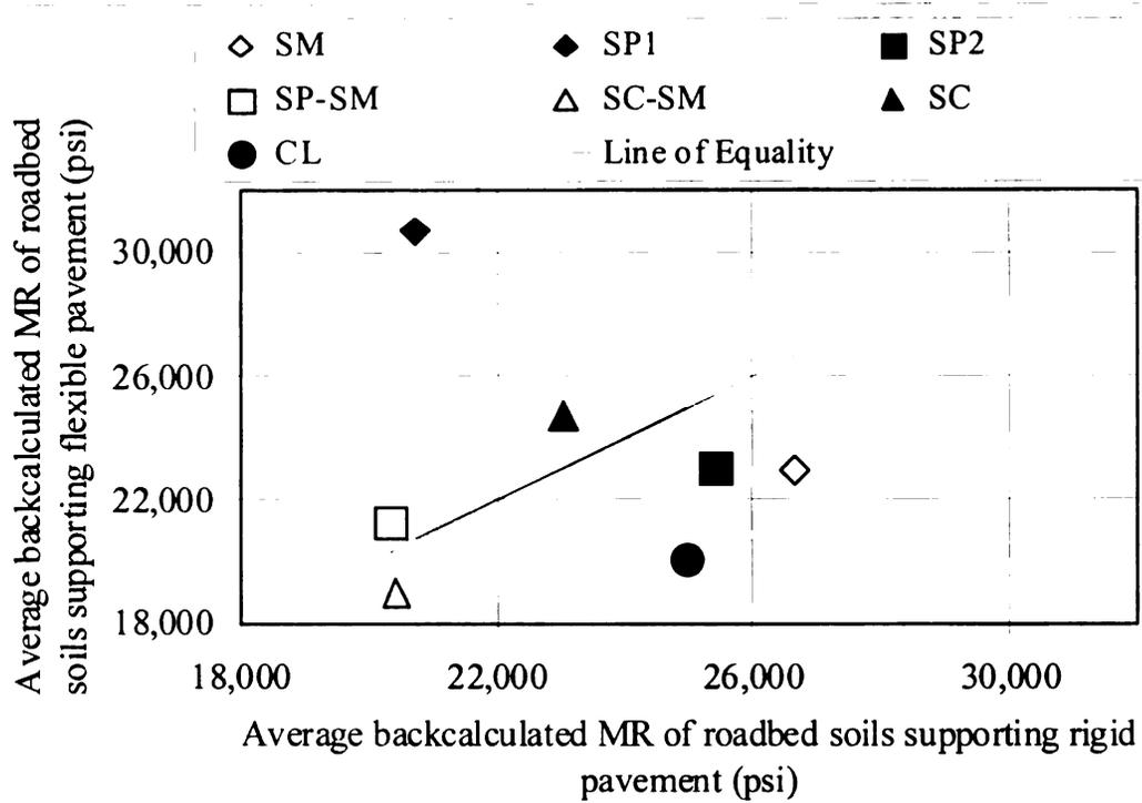
Figure 4.20 Flexible vs. rigid backcalculated roadbed soil MR
