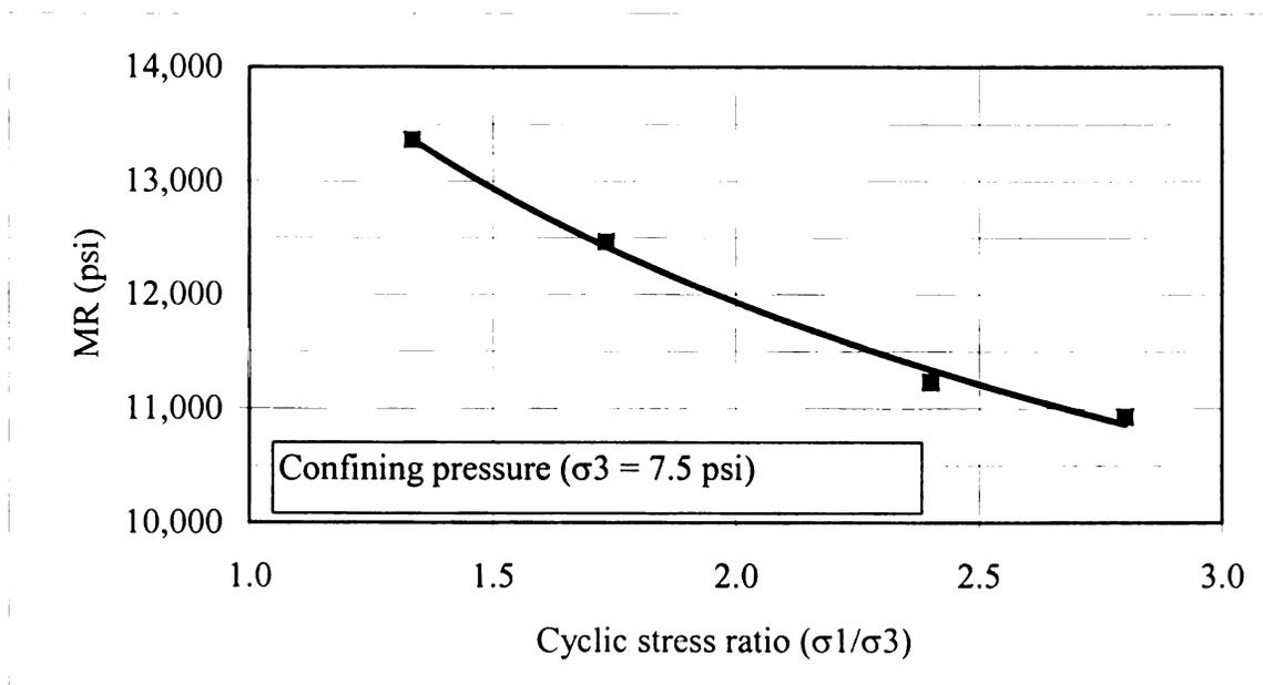
Figure 4.27 Laboratory obtained resilient modulus versus the cyclic stress level
