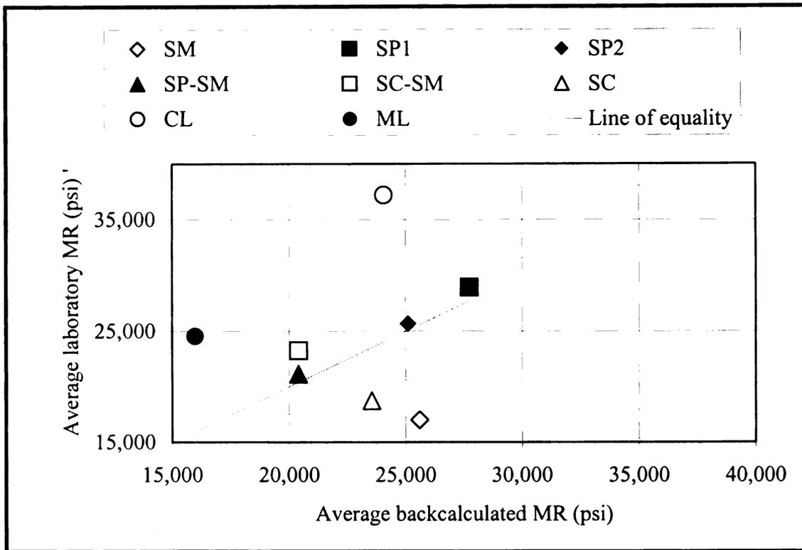
Figure 4.25 Laboratory determined and backcalculated roadbed soil MR
