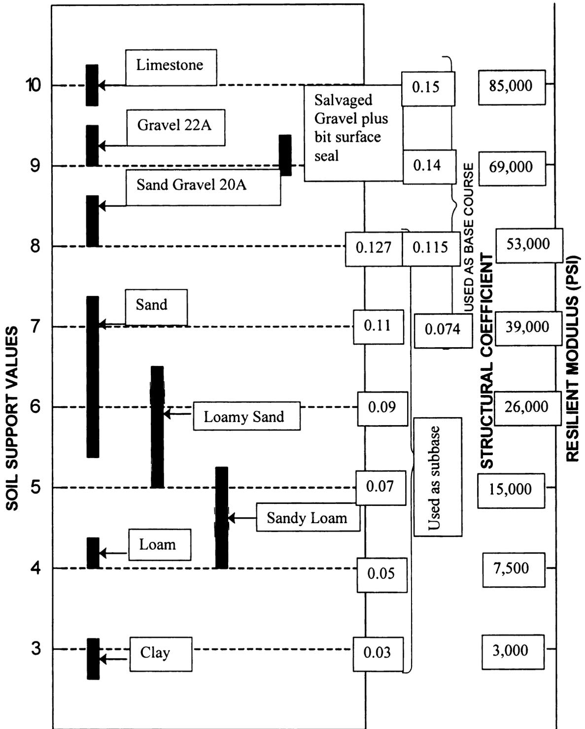
Figure 2.2 Soil support, structural coefficient, and MR correlations (MDSH)
