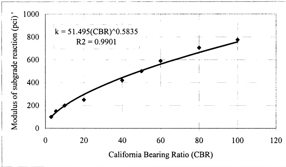
Figure 4.19 Modulus of subgrade reaction versus California Bearing Ratio (after NHI 1998)
