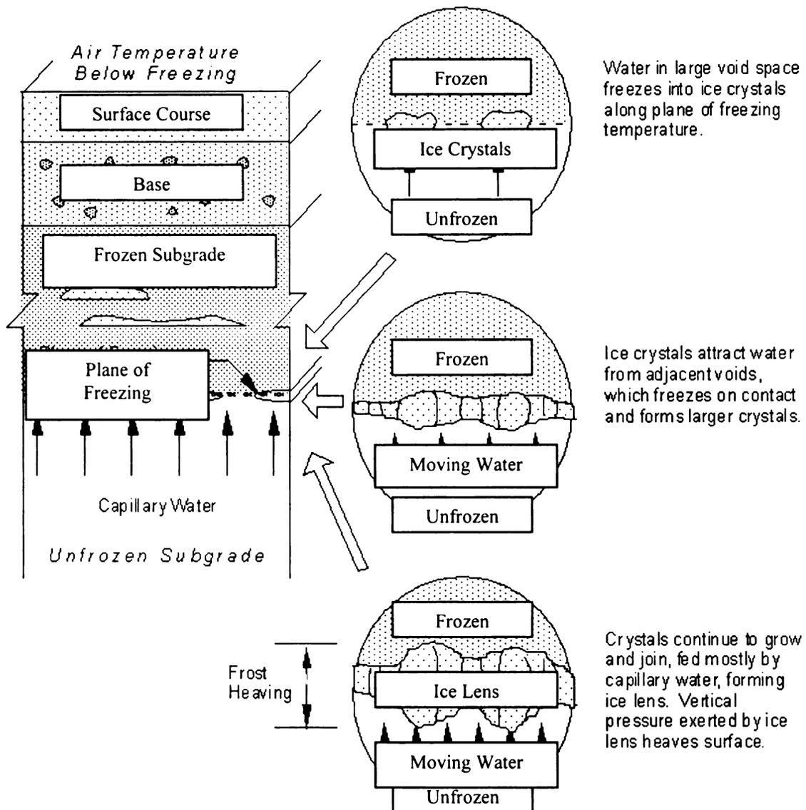
Figure 2.12 Formations of ice lenses in a pavement structure (PTC 2008)
