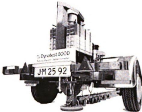
Figure 2.7 Dynatest Falling Weight Deflectometer
