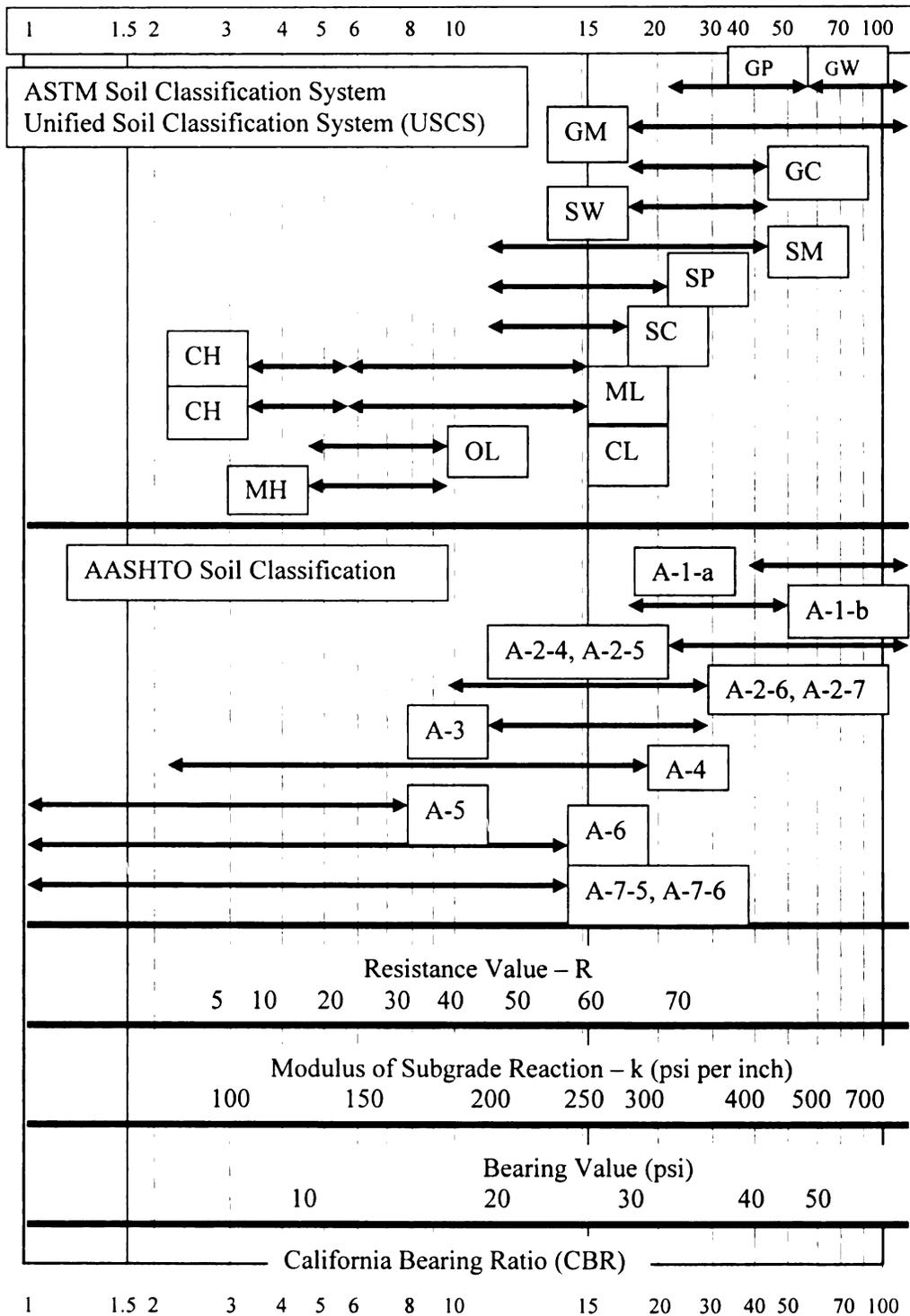
Figure 2.3 Soil classification related to strength parameters (NHI 1998)
