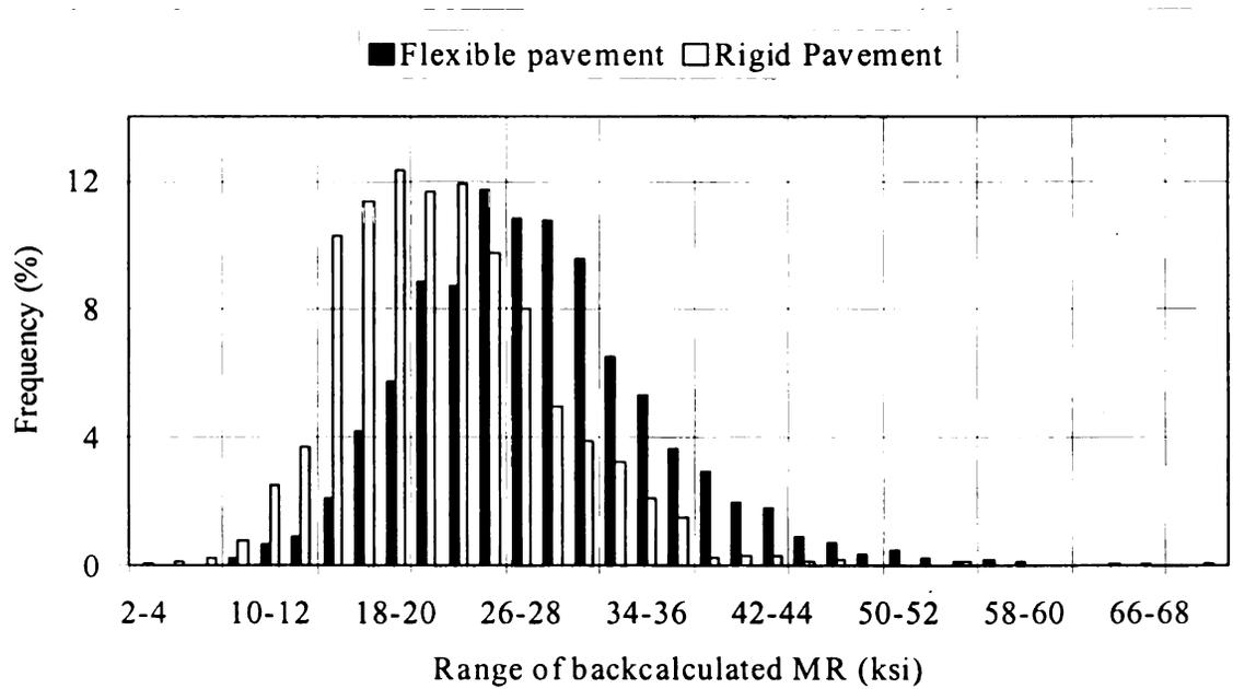
Figure 4.21 Frequency of backcalculated MR of roadbed soils under flexible and rigid pavements
