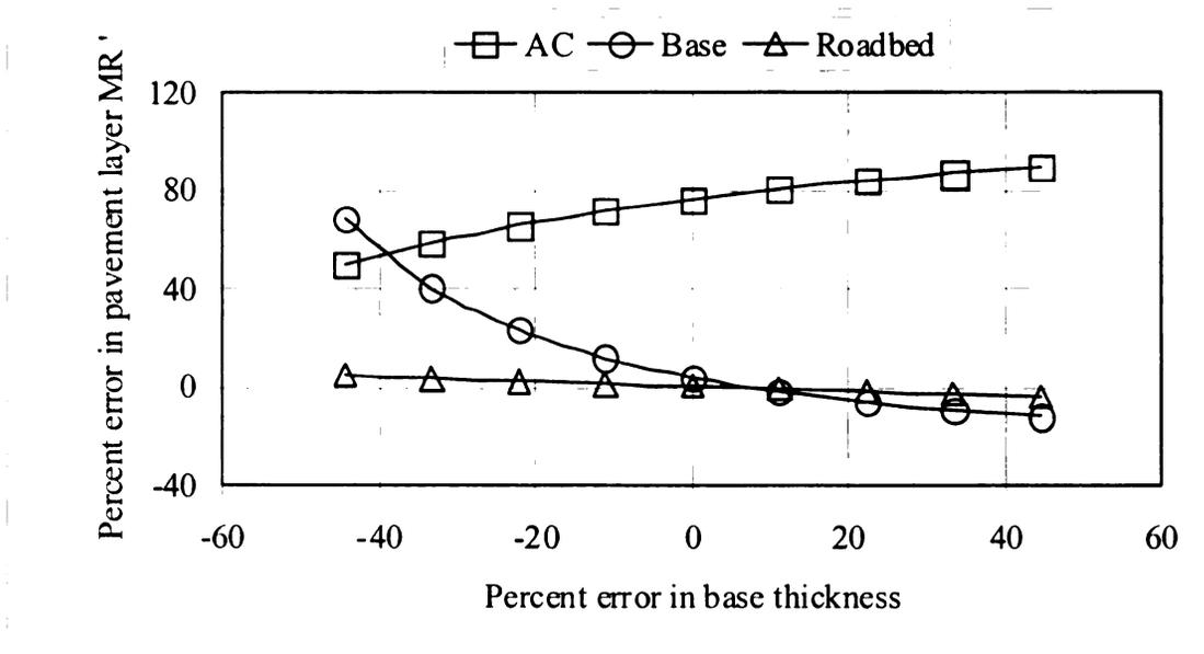
Figure 4.8 Effect of base layer thickness on MR
