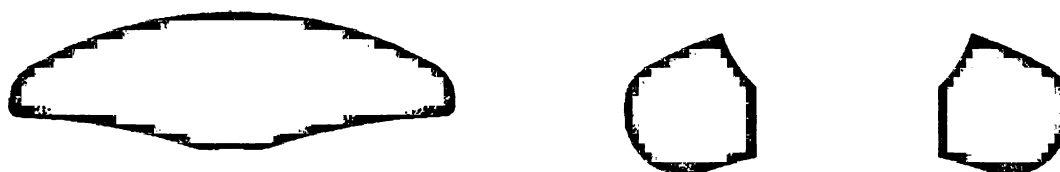
Figure 1-30. Cross-section of the LC-DCP. The figure on the left is the solid section of the plate where the bend occurs; the figure on the right is the section where a hole was present.
