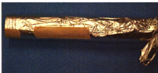
Figure A1-17. Depuy plastic tube with aluminum foil shell.
