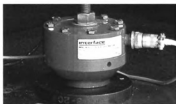
Figure 1-20. 500 lb load cell, mounted on the base of the Instron table.
