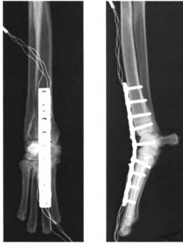
Figure 1-17. Dorsopalmar (left) and mediolateral (right) radiographs of specimen implanted with fully instrumented LC-DCP, MSU SACS
