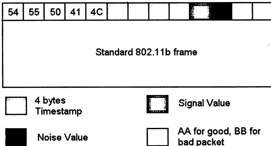
**Figure 3.3 Modified Meta Frame captured by Ethereal**
