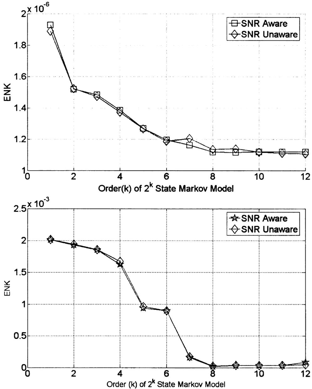
**Figure 4.5 ENK for Burst Length of errors for 11Mbps(Top) and 5.5 Mbps (Bottom) for Office Data**
