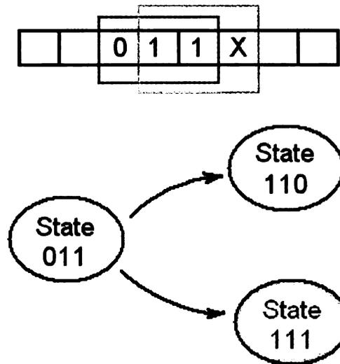
**Figure 4.1 Transition possibilities for sliding window with  $k=3$**
