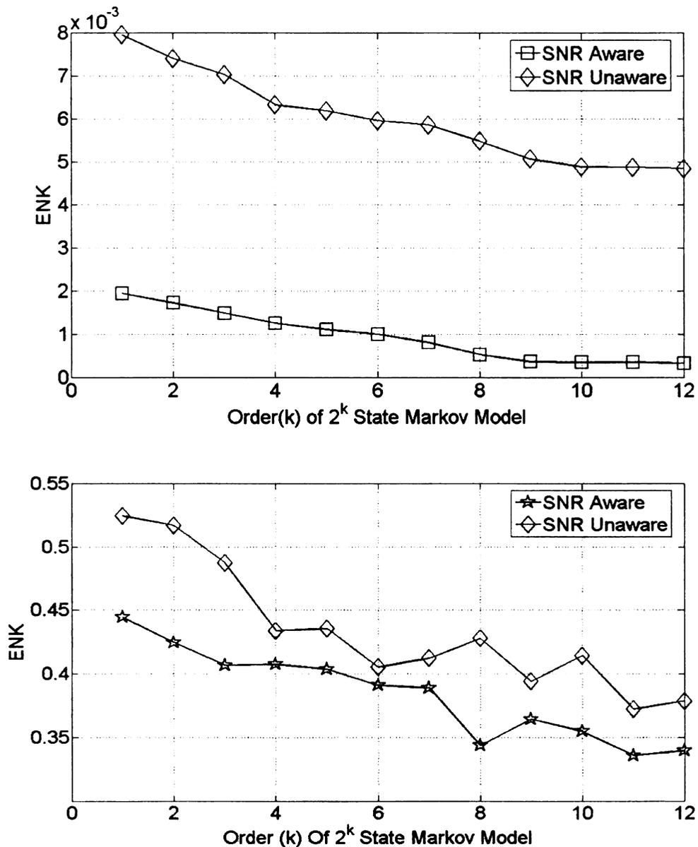
Figure 4.6 ENK for per packet errors for 11Mbps(Top) and 5.5 Mbps (Bottom)
