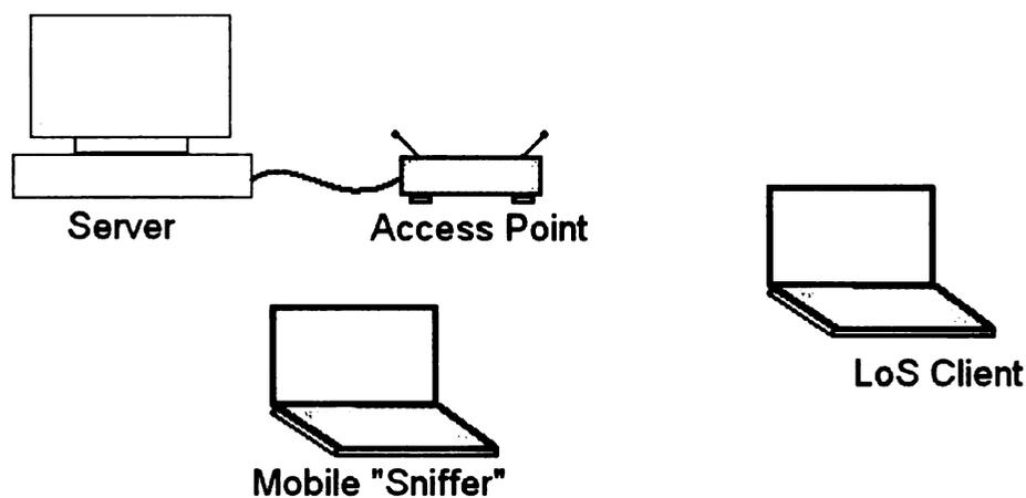
**Figure 3.1 Experimental Setup showing Server, LoS Client and the Sniffer**
