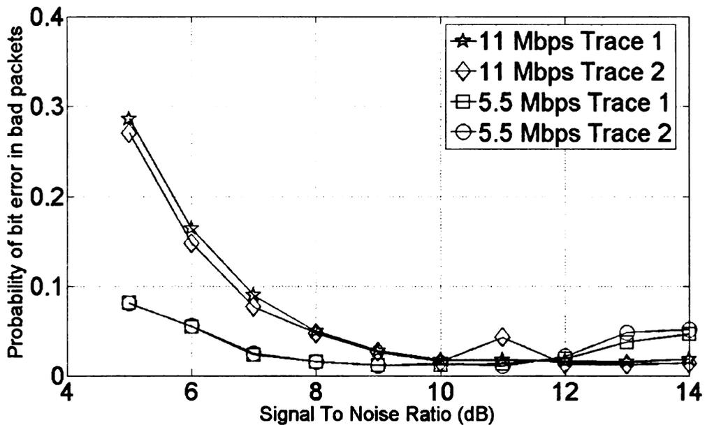
**Figure 3.6 Probability of error ( $p$ ) In bad packets V/S Signal-To-Noise Ratio (dB)**
