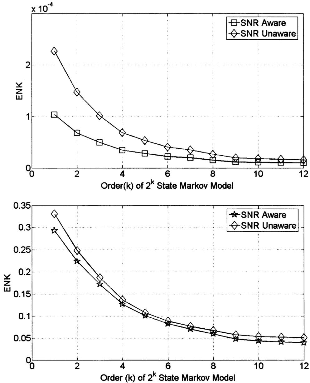
**Figure 4.3 ENK for Inter-Arrival of errors for 11Mbps(Top) and 5.5 Mbps (Bottom) for Office Data**
