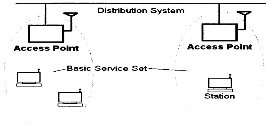
**Figure 2.1 IEEE 802.11 WLAN Extended Service Set**
