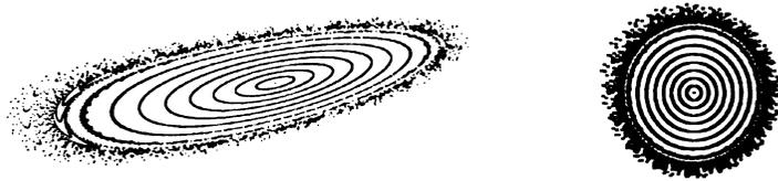
**Figure 1.1:** Phase space trajectories in FODO cell, obtained for 1000 turns by applying one turn map to the vector with initial coordinates 1000 times; in conventional (left) and normal form (right) coordinates
