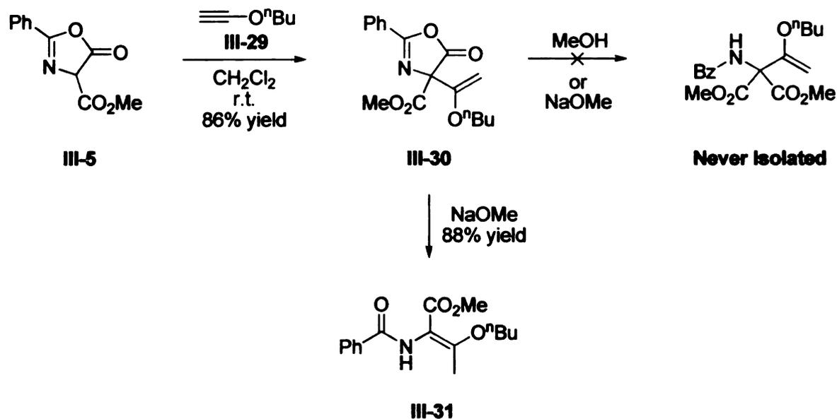
**Scheme III-15.** Reaction of 2-phenyl-4-carbomethoxy-5(4H)-oxazolone **III-5** with 1-butoxyethyne **III-29** followed by methanolysis.
