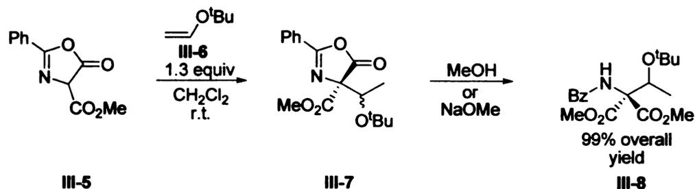
**Scheme III-13.** Intermolecular alkylation of 2-phenyl-4-carbomethoxy-5(4H)-oxazolone III-5 with *tert*-butyl vinyl ether III-6 followed by methanolysis.
