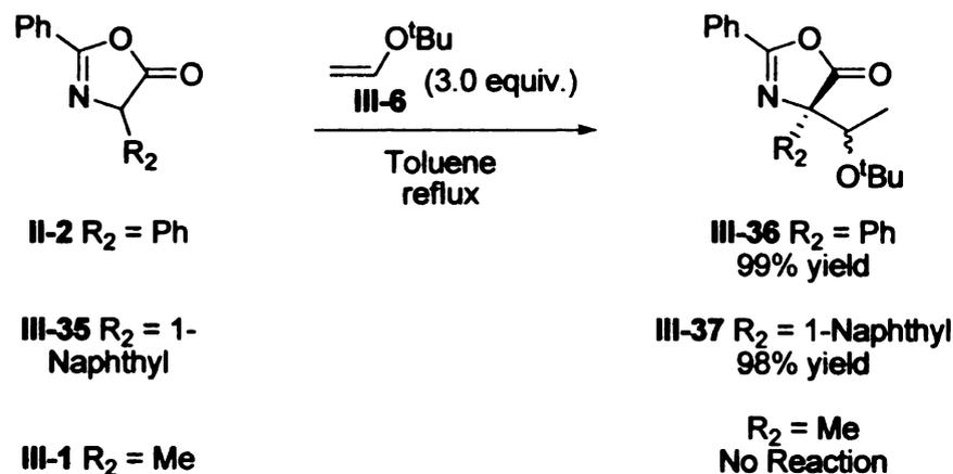
**Scheme III-17.** Reaction of 4-aryloxazol-5(4H)-ones and 4-alkyloxazol-5(4H)-ones with *tert*-butyl vinyl ether **III-6**.
