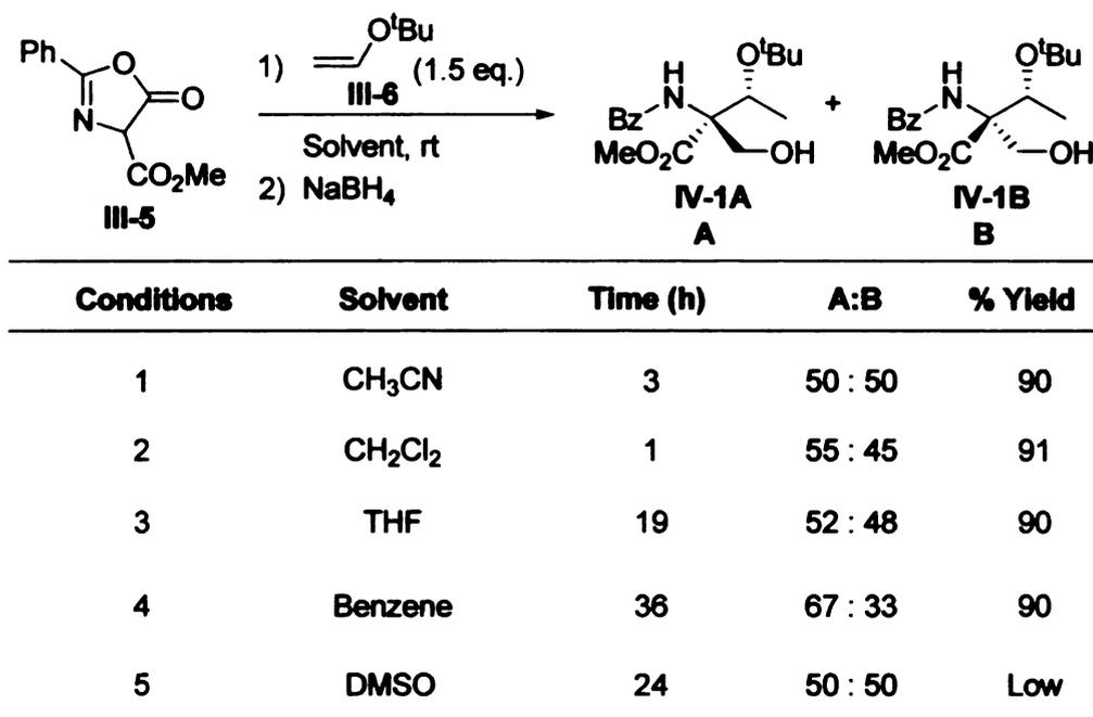
**Table IV-1.** Reaction of 4-carbomethoxy-2-phenyl-5(4H)-oxazolone III-5 with *tert*-butyl vinyl ether III-6 followed by reduction with sodium borohydride.
