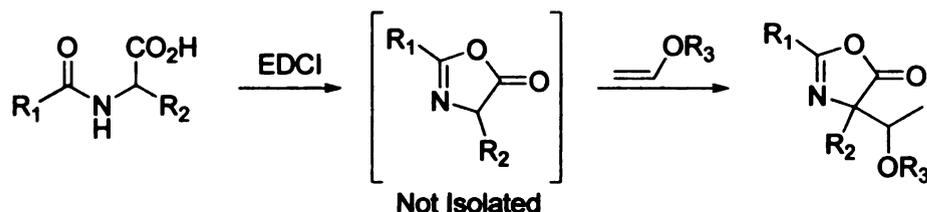
**Scheme III-22.** Conducting the intermolecular alkylation reaction of oxazol-5(4H)-ones with enol ethers while generating the starting oxazol-5(4H)-one *in situ*.
