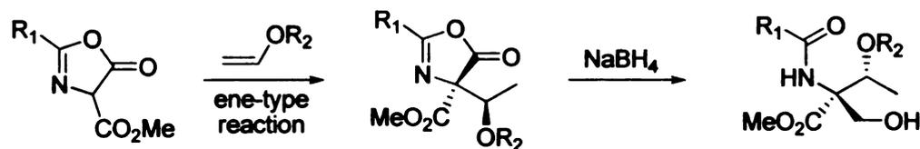
**Scheme IV-7.** Proposed synthesis of *tert*-alkyl amino hydroxy carboxylic acids.
