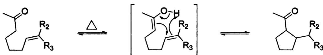
**Scheme III-10.** General thermal Conia-ene cyclization.
