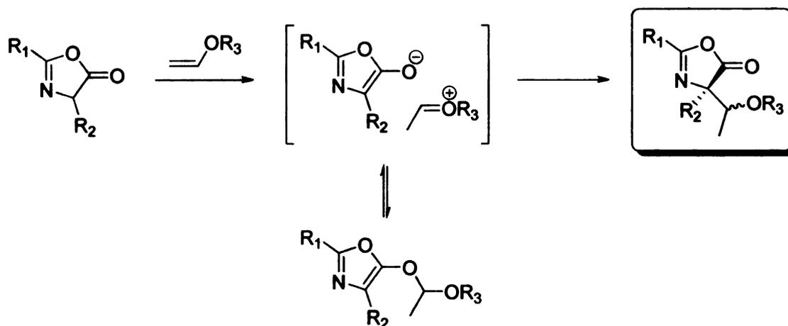
**Scheme III-21.** Current mechanistic understanding of the alkylation of oxazol-5(4H)-ones with enol ethers.
