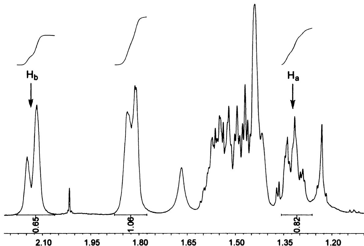
**Figure III-5.** <sup>1</sup>H NMR spectra of the product mixture obtained from treatment of oxazol-5(4H)-one III-5 with enol ether III-38 containing 50% deuterium.
