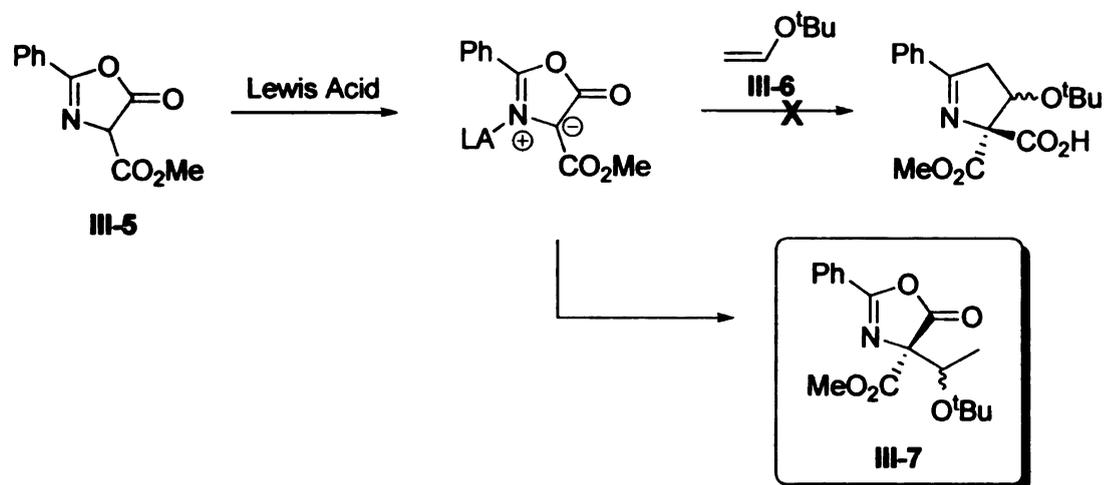
**Scheme III-8.** Reaction of 2-phenyl-4-carbomethoxy-5(4H)-oxazolone III-5 with *tert*-butyl vinyl ether III-6 to form the quaternary substituted oxazolone III-7.
