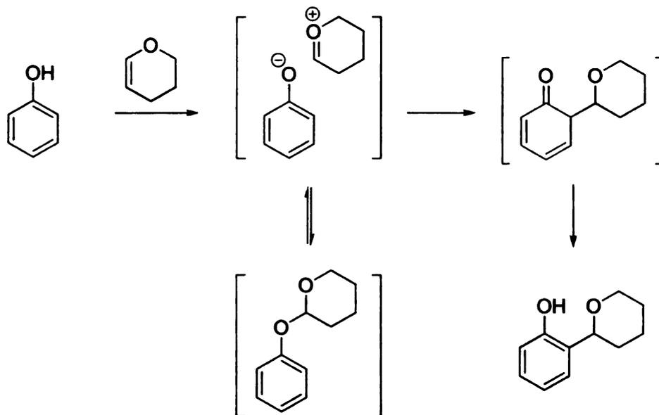
**Scheme III-12.** The thermal ortho-alkylation of phenols using enol ethers.
