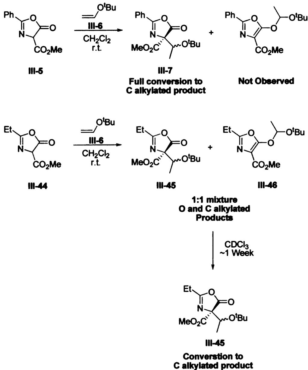
**Scheme III-20.** Comparison of the reactivity of 2-phenyl-4-carbomethoxy-5(4H)-oxazolone **III-5** and 2-ethyl-4-carbomethoxy-5(4H)-oxazolone **III-44**.
