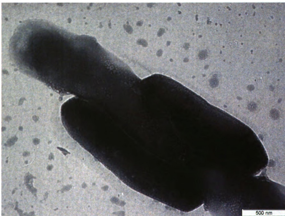
Figure 4.16 TEM image of the nanocomposite and Rhizobium trifolii sample, showing four cells coated with nanocomposite.
