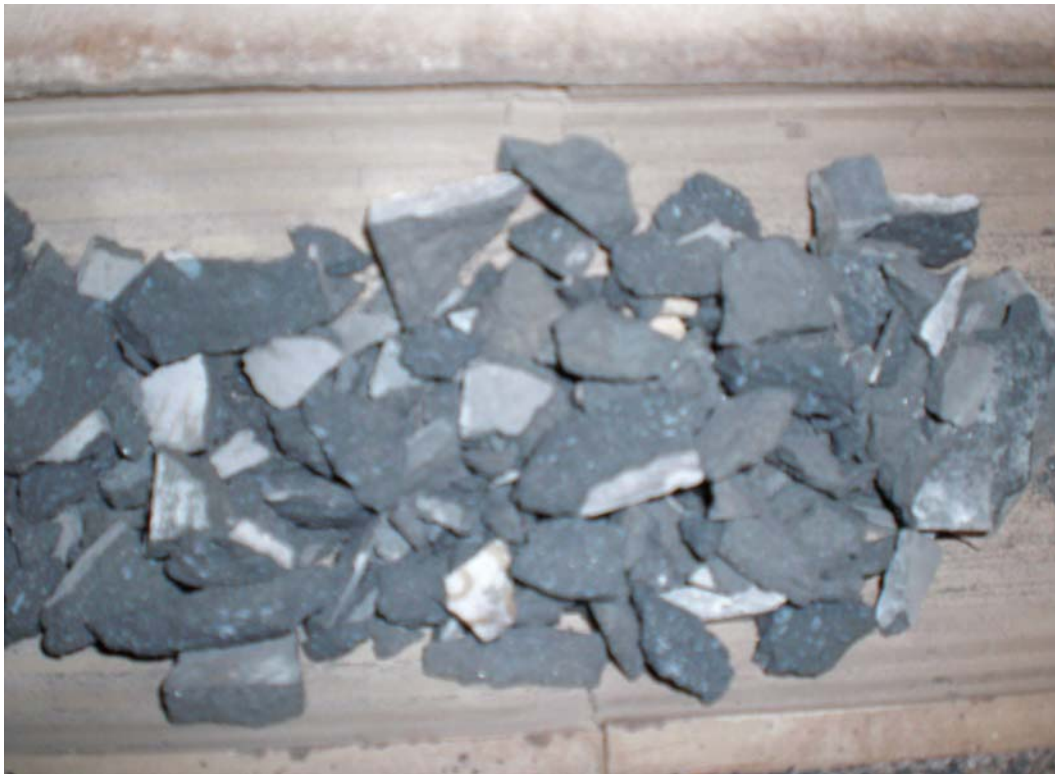
(a) Failed plain DSP mortar specimens
