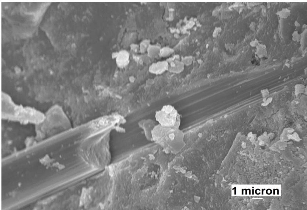
(b) Failure mechanism of micro-scale fibers at fracture surfaces
