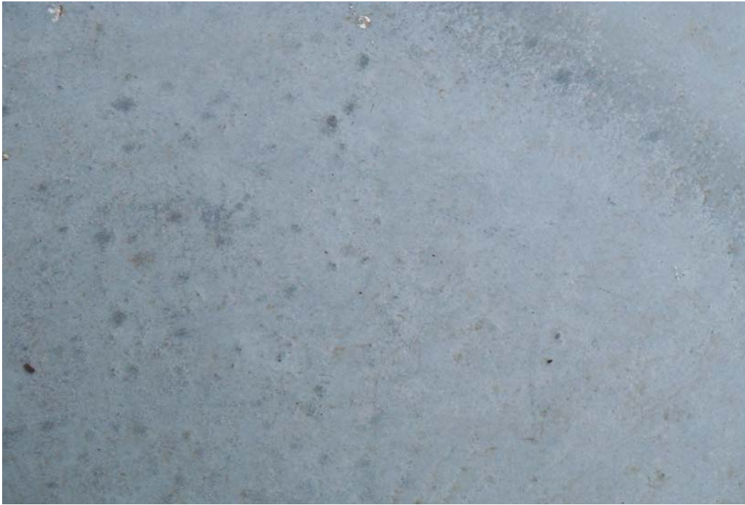
(g) Finished look of HSC nanocomposites after 3 months
