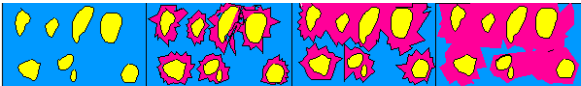
(a) Hydration of cement particles partially filling the space between them
