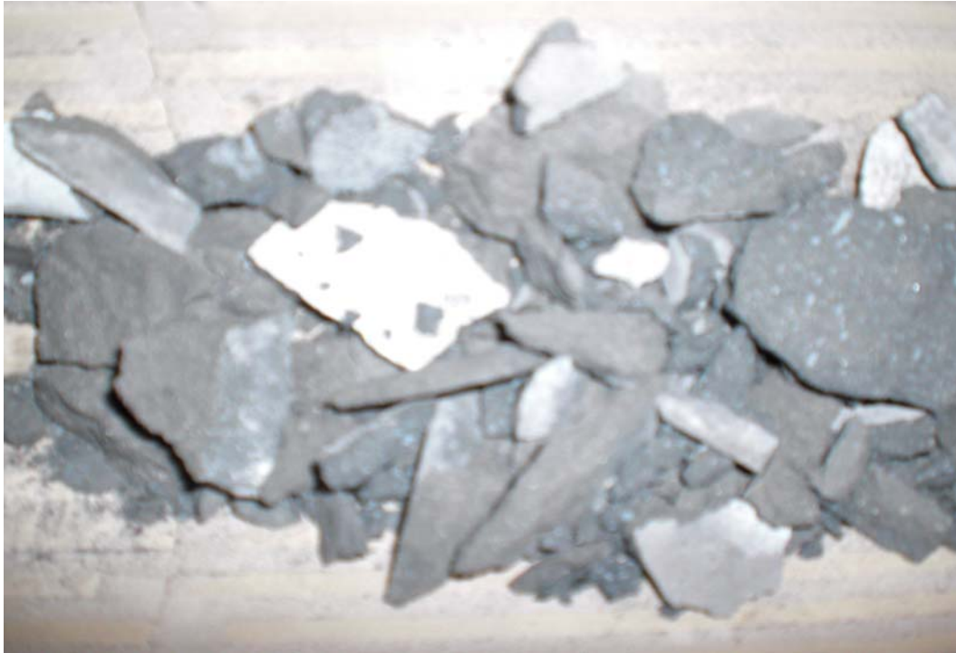
(a) Failed DSP mortar with hybrid reinforcement
