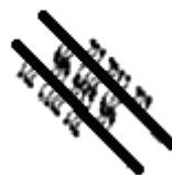
Figure 2.5- Steric and electrostatic repulsion of separated nanotubes.
