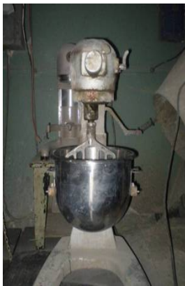
(a) Mortar Mixer
