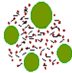
(b) CNT in cement (left) & cement/silica fume (right)
