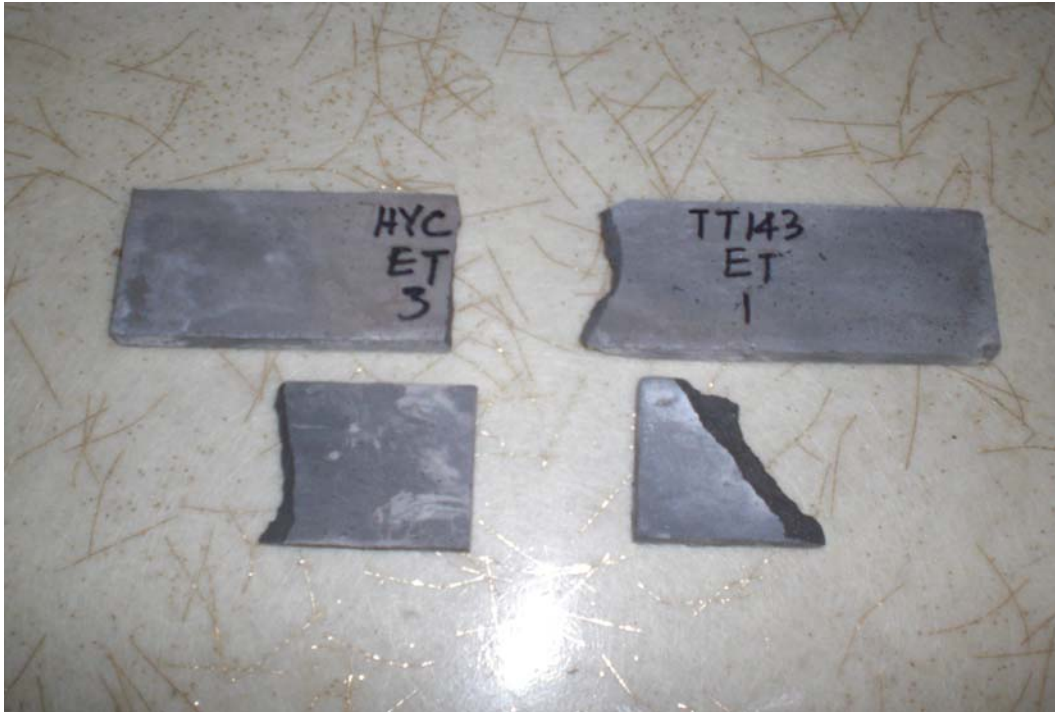
(b) Failed DSP mortar with hybrid reinforcement
