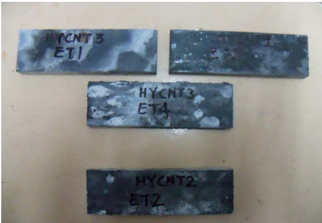
(b) Survived DSP mortar with hybrid reinforcement
