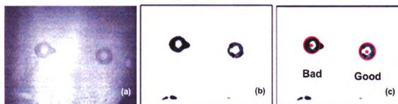
Figure 5.10 Three-step characterization for surface interior MO images (a) raw images (b) enhanced images using motion-based filtering (c) detection and classification of images
