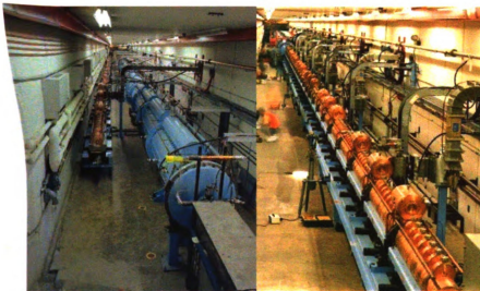
Figure 2.4: A picture of Fermilab's Linac. On the left is shown the drift tube Linac whereas on the right is shown the high energy part of the Linac. Both of the components make up the Linac. H^- ions enter the Linac at the drift tube side of the Linac.
