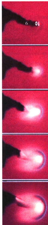
Figure 10-1. A single flamelet (~6 mm wide) propagates steadily in an air flow of 0.5 cm/s in the NASA NCA. When the air flow is abruptly increased to 50 cm/s (100x), the flamelet grows 200% in less than 10 seconds. (Each photograph is 2 sec after the preceding one) [155].
