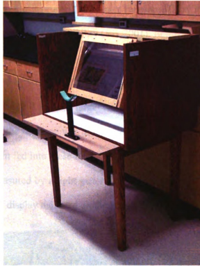
Figure 11 - Custom Designed Eye Tracking Table with Glass pane and Chin rest arrangement
