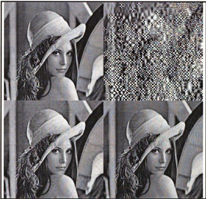
Figure 7.4. JPEG2000 encoded 'lenna' image with (clockwise from left) i- original image after source encoding ii- end-to-end channel coding with  $\epsilon = 0.07$  iii- PERA with  $\epsilon = 0.18$  iv-D-OPERA with  $\epsilon = 0.143$
