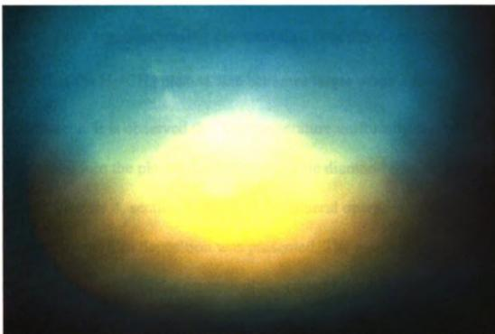
Figure 5-7: A photograph of the heated substrate without using any groove-patterned inserts. Usually the center of the substrate is hotter than the edge.
