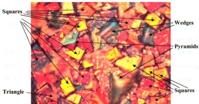
Figure 3-27: The surface morphology of diamond film sample SZ-2inch-1mm-035. Most crystal surface shows a square shape of facet with a few grains show part of the grain tips look like pyramids or wedges.
