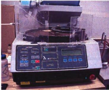
Figure 3-30: Logitech LP 50 lapping and polishing system.
