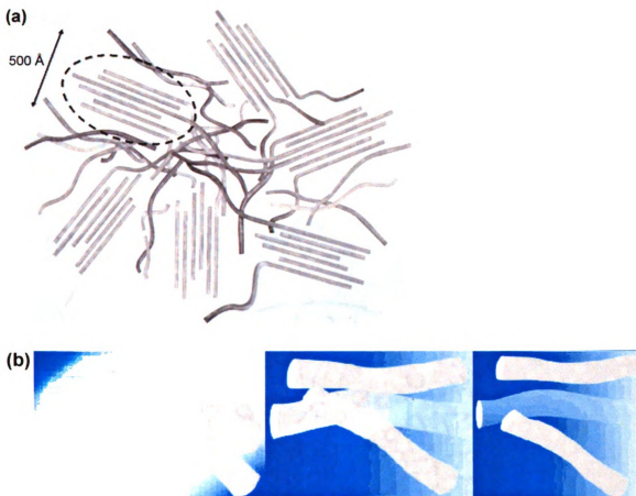
Figure 3. Polymer-bundle model. (a) Schematic view of polymer aggregate domains inside a bundle. (b) Schematic view of nanoscopic swelling between three polymer aggregates inside a bundle with different water contents. (from almost dry membrane (left) up to diluted solution (right)). (Reprinted with permission from Macromolecules 2004 , 37 , 7772-7783. Copyright 2004 American Chemical Society)
