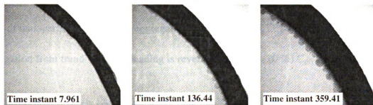
Figure 2.2. Schematic (A) of an isothermal phase diagram for a three component (solvent-polymer-nonsolvent) system and laser-scanned brightfield images (B) of demixing front propagation in PSf-C 60 -PVP-NMP blends as a function of time (in seconds) of exposure to nonsolvent (water).
