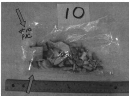
The PVC fragments of pipe bomb #10 being prepared for soaking. The plastic pouch was constructed by heat-sealing the top and bottom of the bag (arrows). The sides were pre-sealed by the manufacturer.
