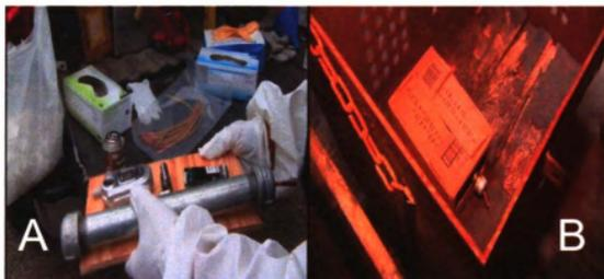
Fuses were inserted into the pipes through the end cap holes and the bombs were clipped onto the detonation devices using the metal clamps (A). The bombs and detonation devices were placed into the carrying containers and put into the metal box to be deflagrated (B).
