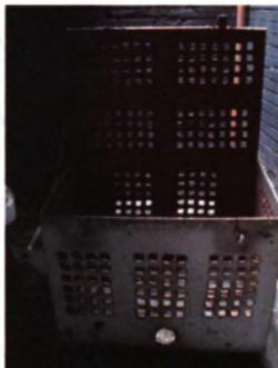
The metal box was supplied by the Michigan State Police bomb squad. Its purpose was to reduce the scatter of the pipe fragments upon deflagration, so that they could be easily collected. Ventilation holes were cut into the sides and lid so that the pressure from the blast could be released.
