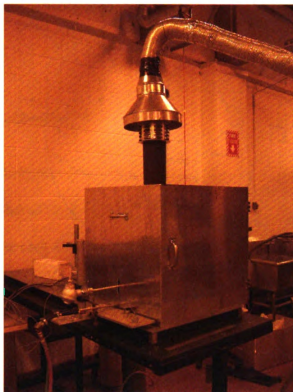
Figure 8: View of the outside of the flame box showing the vent, door, thermocouple, and torch.
