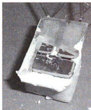
Figure 202: After the module dropped 9' the base aluminum nitride cracked.
