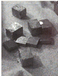
Figure 90: Picture of failed bonds of Bi 2 Te 3 to the LAST material.
