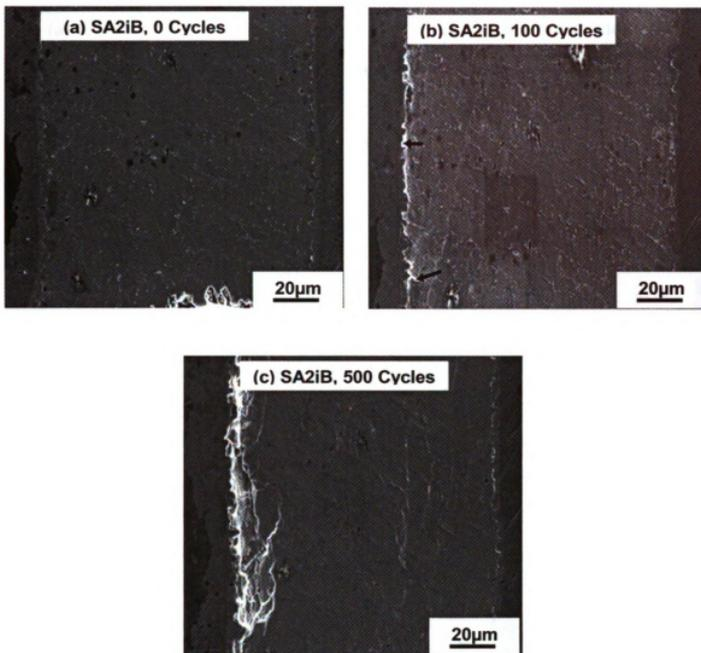
**Figure 4.3.3** SEM images showing surface damage evolution in SA + 2wt% Iso-Butyl trisilanol (SA2iB) solder joint due to low temperature regime TMF between  $-55^{\circ}\text{C}$  to  $125^{\circ}\text{C}$ . Surface damages after 100 cycles of TMF has been indicate with arrows.
