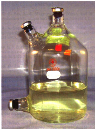
Figure B.2. Black butyl rubber stoppers with crimped aluminum seals on a specially designed 3-port 1 l flask. These 3-port flasks were used to hold maximally 500 ml anaerobically.
