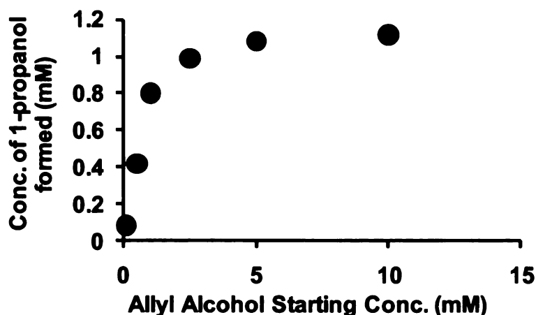
Figure 3.11 Concentration of 1-propanol formed in membrane-catalyzed hydrogenation with several initial allyl alcohol concentrations. Solutions were sparged with H_2 , and the flux through the Pd nanoparticle-modified alumina membrane was 0.023 mL/cm 2 -sec.
