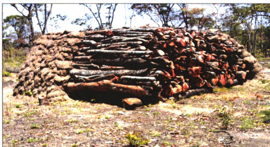
Figure 37. Earth Kiln Partly Covered with Earth, 2007
