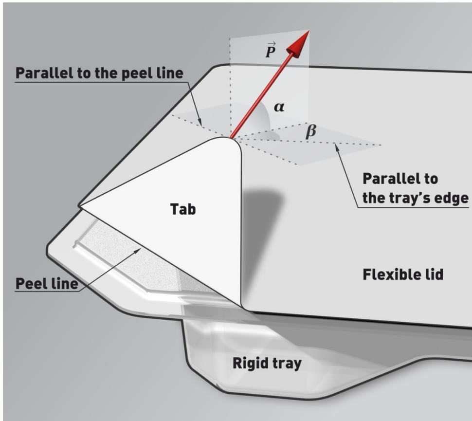
**Figure 4.1** – Peel force and peel angles of a tab.
