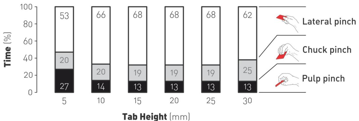
**Figure 7.9** – Proportion of time spent on each grip during pulling for each tab size.
