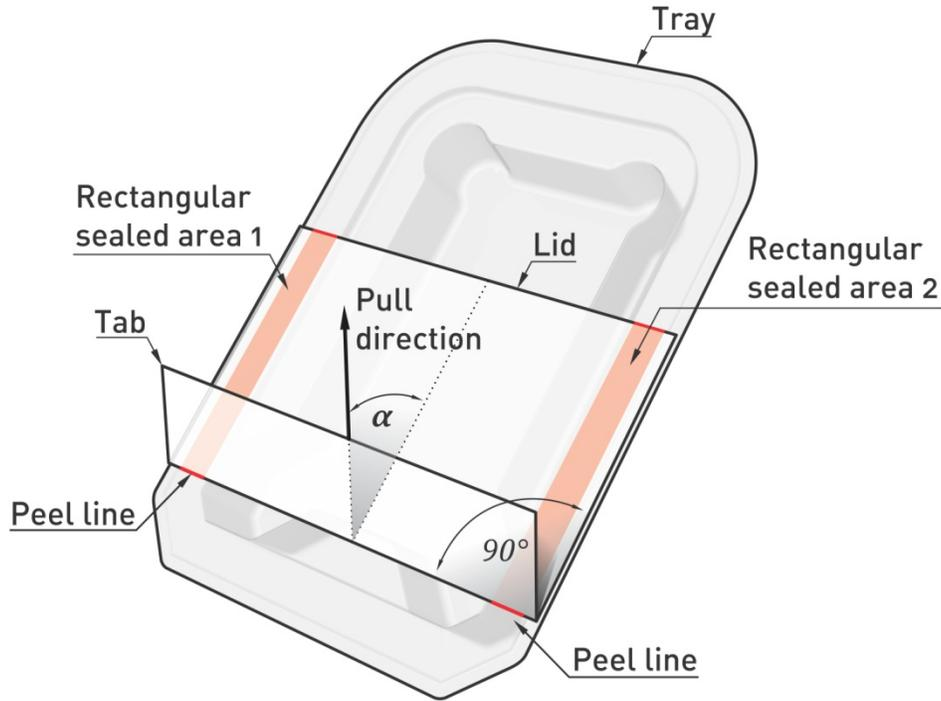
**Figure 4.4** – Condition B: Partially lidded tray with two rectangular sealed areas (in red) tested at  $\beta=0^\circ$  and  $\alpha=0-90^\circ$  (shown at  $\alpha=45^\circ$ ).
