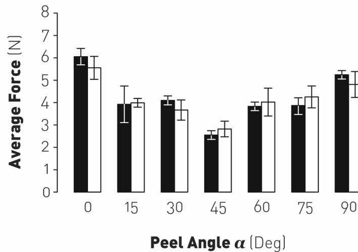
**Figure 5.6** – Comparison of experimental and theoretical average forces at various peel angles. Experimental (■); Theoretical values calculated using average seal strength (□).
