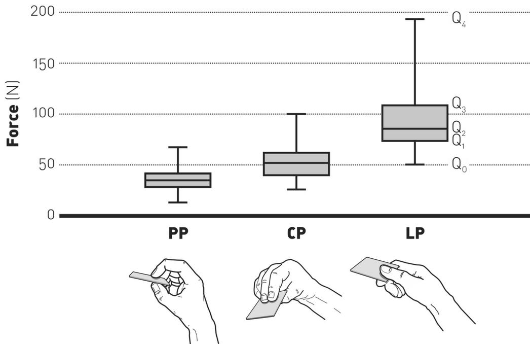
**Figure 7.2** – Box-plots of pull-tear forces for three types of pinch.
