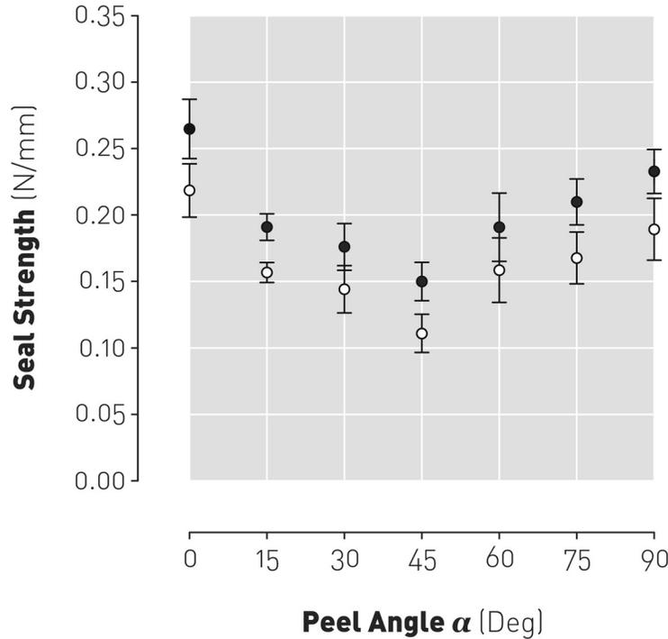
**Figure 5.3** – Peak (●) and average (○) seal strength vs. peel angle.
