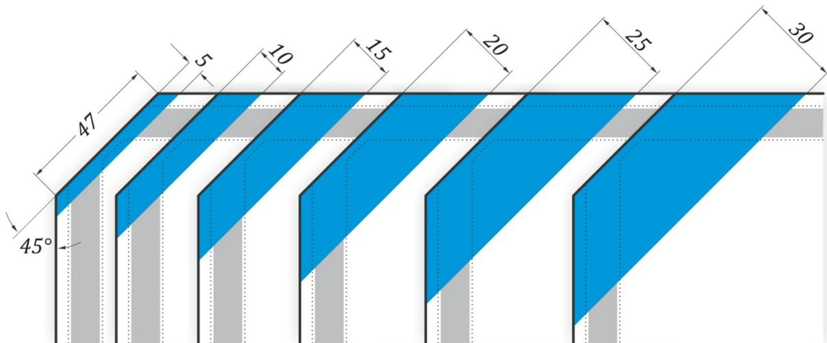
**Figure 7.4** – Tab dimensions in mm.
