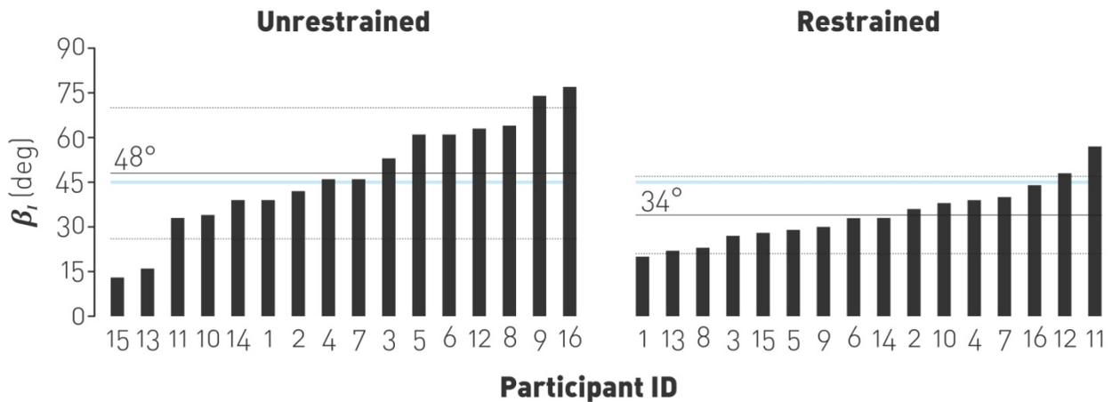
**Figure 6.13** – Average initial peel direction angle ( $\beta_I$ ) for each participant in both experimental setups. The horizontal lines represent the mean peel angle and one standard deviation from it. The blue line represents the optimal peel direction angle ( $\beta=45^\circ$ ) at the beginning of the opening task.
