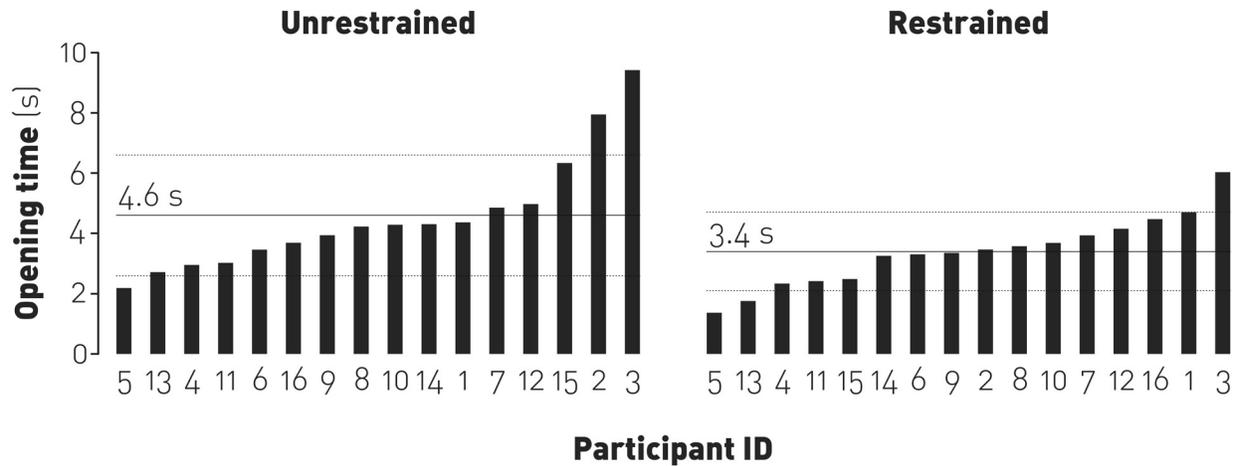
**Figure 6.11** – Average opening time for each participant in both experimental setups. The horizontal lines represent the mean opening time and one standard deviation from it.
