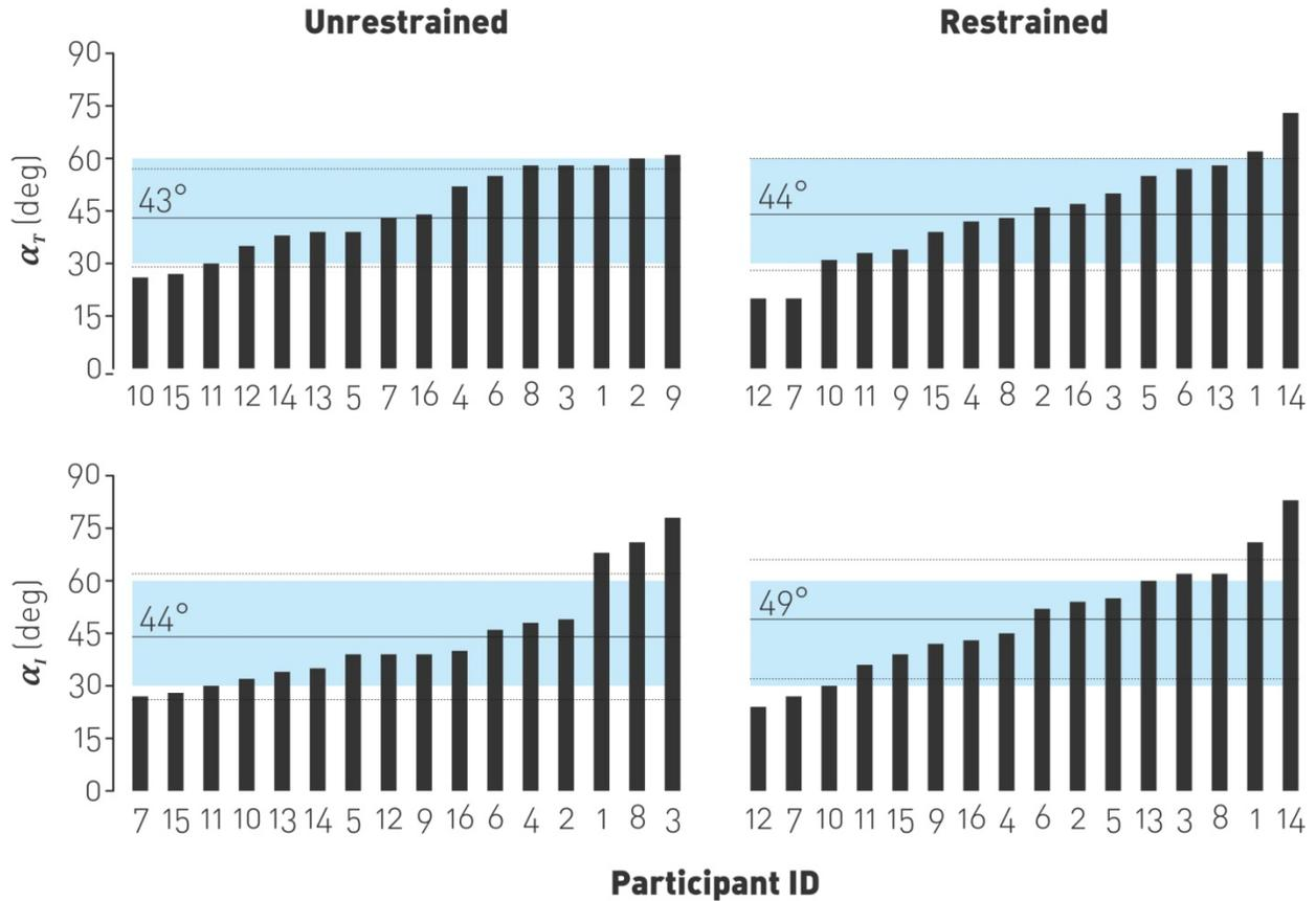
**Figure 6.12** – Average total peel angle ( $\alpha_T$ ) and average initial peel angle ( $\alpha_I$ ) for each participant in both experimental setups. The horizontal lines represent the mean peel angle and one standard deviation from it. The blue area represents the optimal peel angle range ( $\alpha = 45^\circ \pm 15^\circ$ ).
