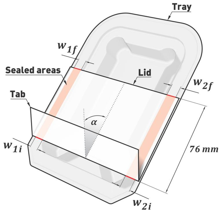
**Figure 5.2** – Rectangular sealed areas (in red) of a tray inclined at  $\alpha=45^\circ$ .
