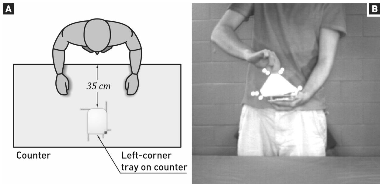
**Figure 6.4** – Unrestrained opening task: (A) Top view of the experimental setup, (B) Participant opening a “left-corner” tray.
