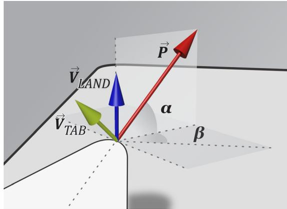
**Figure 6.6** – Angles and vectors involved in the computation of peeling direction.
