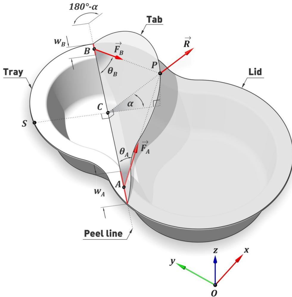
**Figure 5.1** – System of forces in a semi-rigid packaging system.
