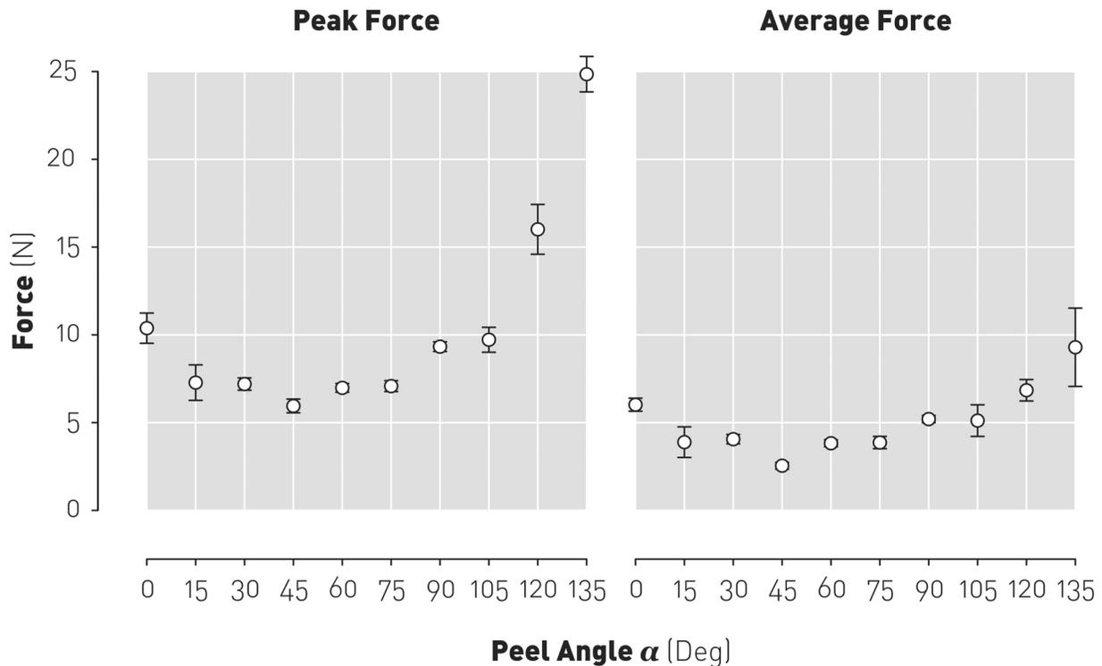
**Figure 4.8** – Condition A: Mean force *vs.* peel angle  $\alpha$ .
