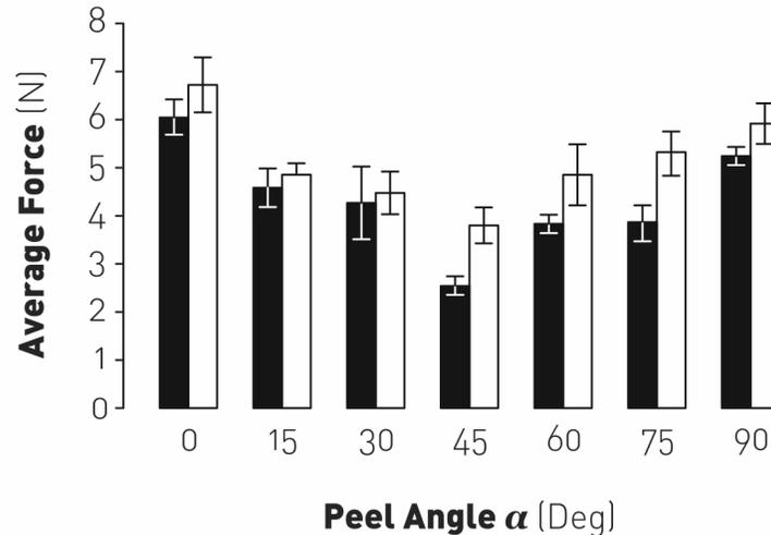
**Figure 5.7** – Comparison of experimental and theoretical average forces at various peel angles. Experimental (■); Theoretical values calculated using peak seal strength (□).
