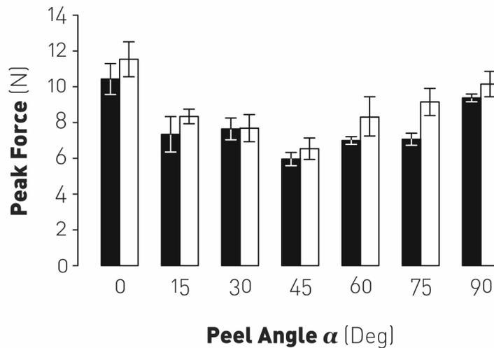
**Figure 5.9** – Comparison of experimental and theoretical peak forces at various peel angles. Experimental (■); Theoretical values calculated using peak seal strength (□).
