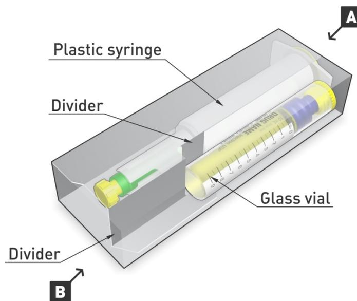
**Figure 3.6** – Internal component’s layout. Notice the two vertical dividers blocking the access of the contents in one end (B). (Note: Text on the vial is irrelevant).
