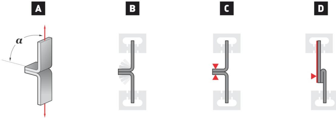
**Figure 4.2** – ASTM F88 sample and tail holding methods: A) Seal sample schematic, B) Unsupported, C) Supported  $90^\circ$ , D) Supported  $180^\circ$ . [1]
