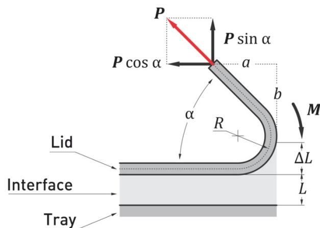
**Figure 4.10** – Theoretical system of forces acting at the peel line.
