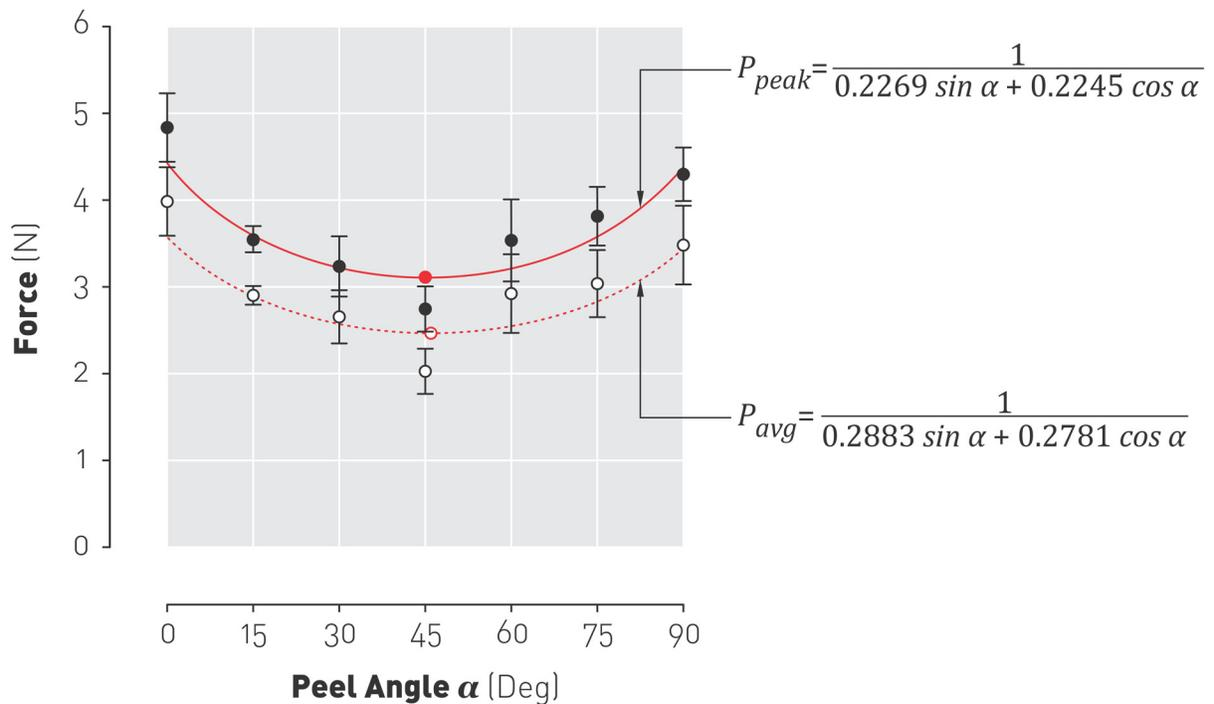
**Figure 4.12** – Condition B: Fitted curves over 0-90° range and experimental data for peak (●) and average (○) forces.
