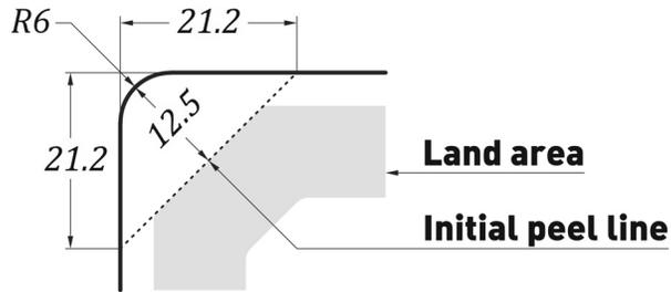
**Figure 6.2** – Tab dimensions in mm, tab’s surface area 217 mm<sup>2</sup>.
