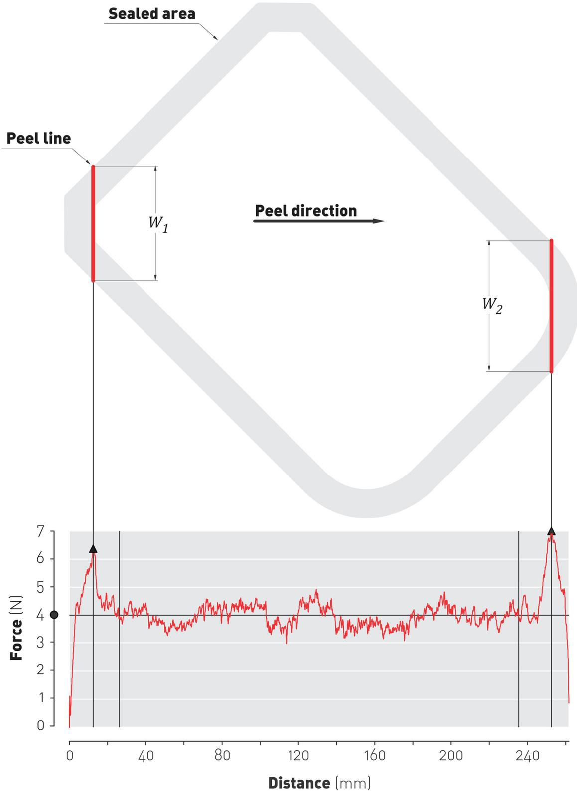
**Figure 4.7** – Condition A: Relationship between peak forces and peel line widths ( $W_1$  and  $W_2$ ).
