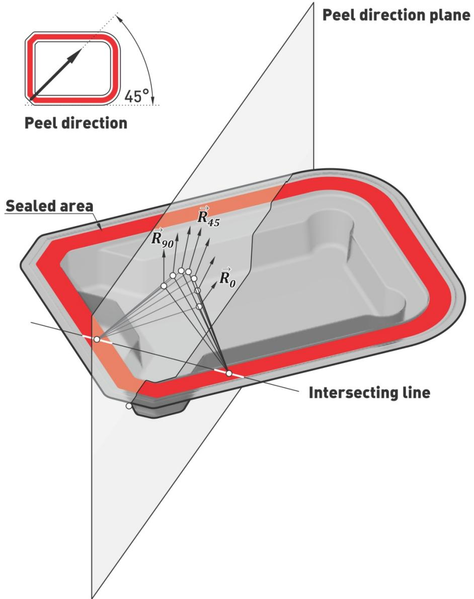
**Figure 5.4** – Sealed area with constant width and peel direction at 45° with respect to the longer tray's edge.
