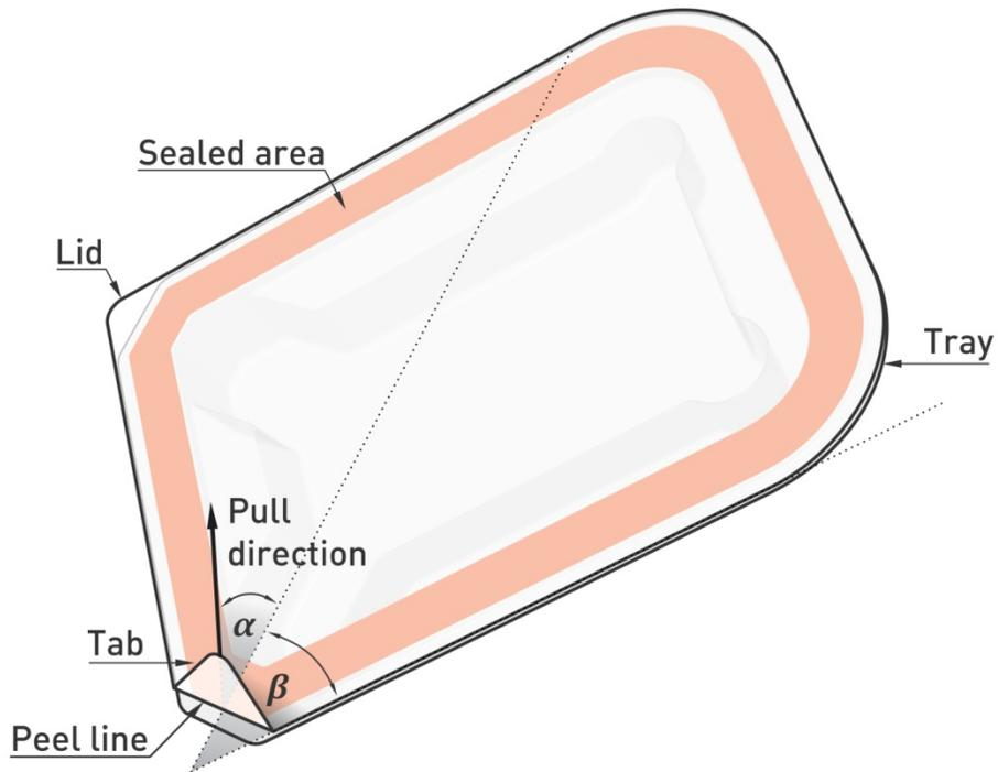
**Figure 4.3** – Condition A: Lidded tray tested at  $\beta=45^\circ$  and  $\alpha=0-135^\circ$  (shown at  $\alpha=45^\circ$ ). Sealed area shown in red.
