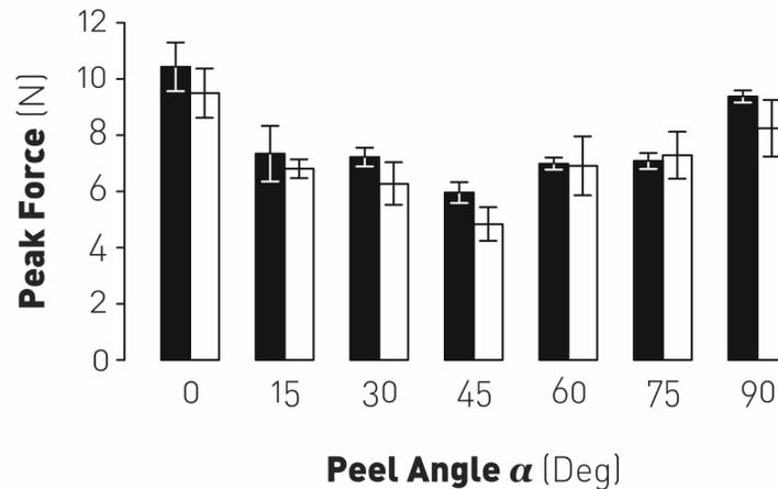
**Figure 5.8** – Comparison of experimental and theoretical peak forces at various peel angles. Experimental (■); Theoretical values calculated using average seal strength (□).
