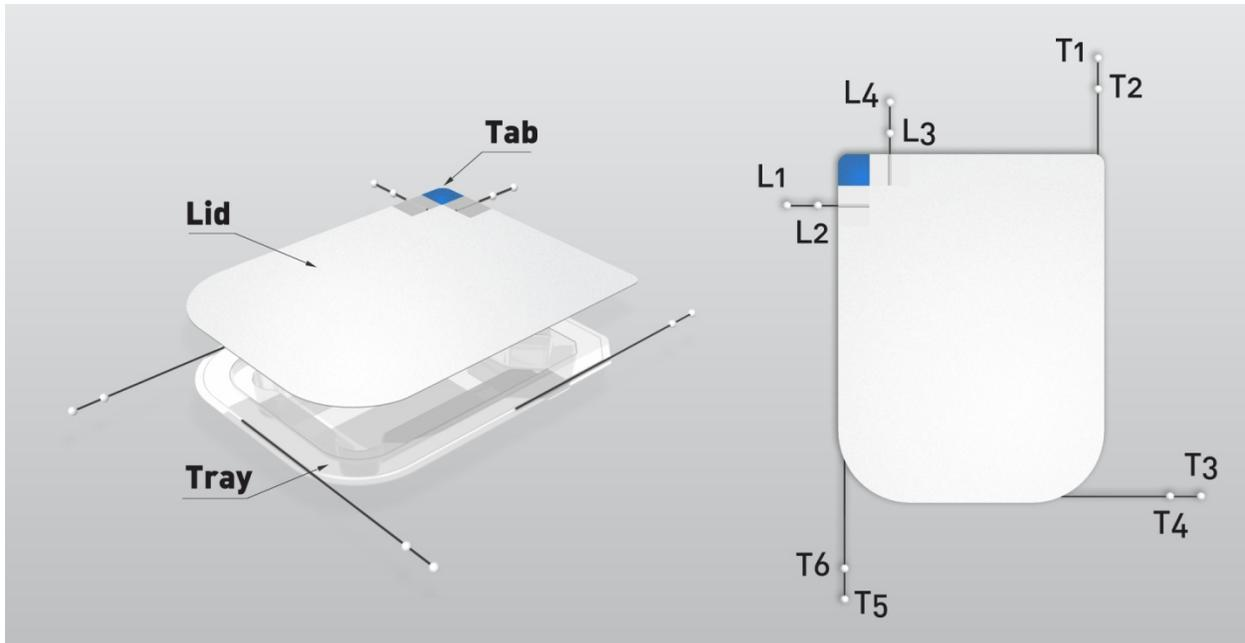
**Figure 6.3** – Placement of the 10 retro-reflective markers for a “left-corner” tray configuration.
