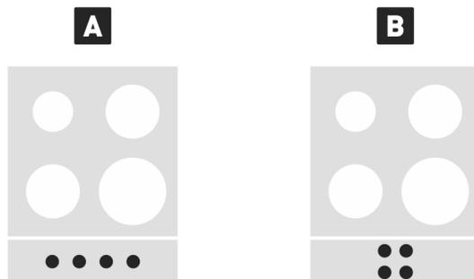
**Figure 3.2** – Logical constraints for stove controls: which knob controls what burner?
