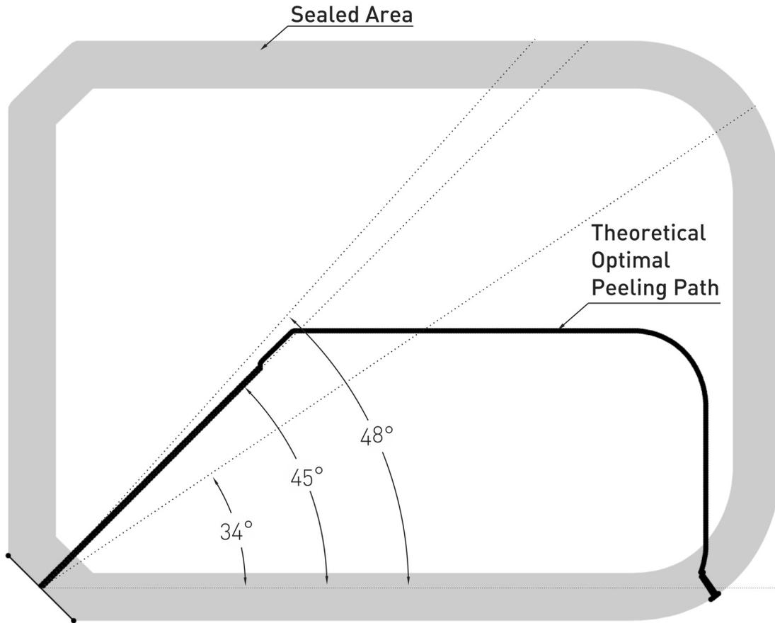
**Figure 6.14** – Comparison of initial peel direction angle ( $\beta_I$ ) for the restrained condition ( $\beta_I = 34^\circ \pm 13^\circ$ ), unrestrained condition  $\beta_I = 48^\circ \pm 22^\circ$ , and the theoretical optimal peeling path ( $\beta_I = 45^\circ$ ).
