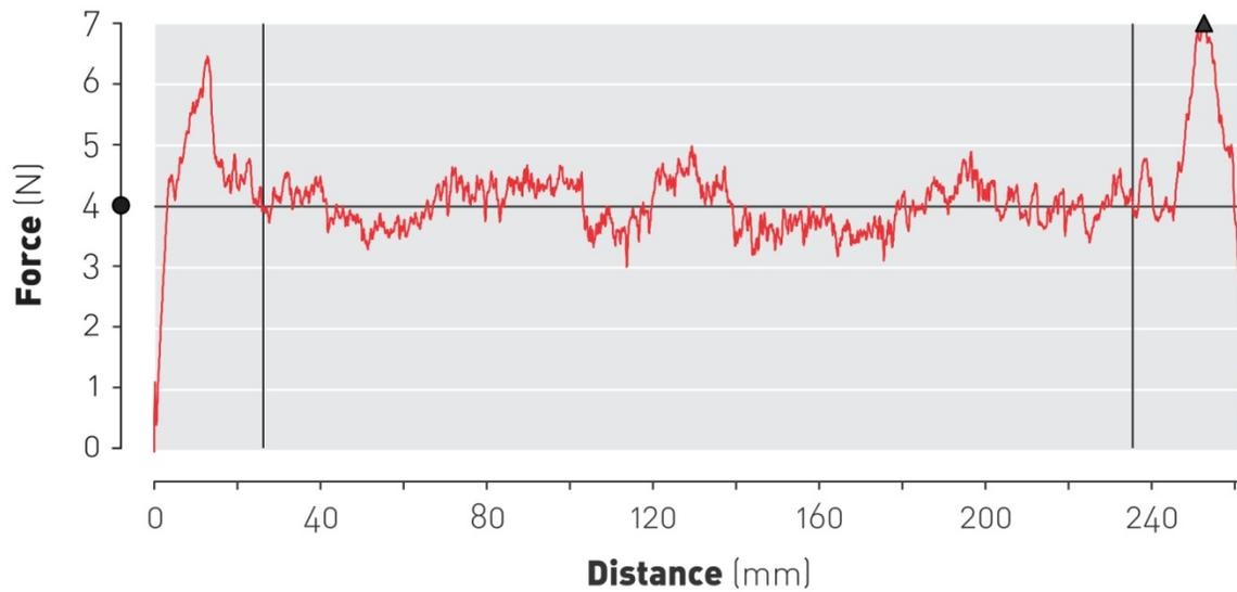
**Figure 4.6** – Example of a Force *vs.* Distance plot for a tray opened at  $\alpha=60^\circ$  and  $\beta=45^\circ$ . ( $\blacktriangle$ ) Peak force, ( $\bullet$ ) Average force.
