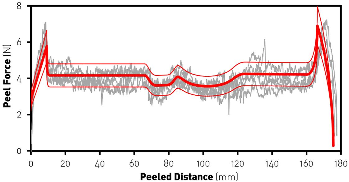
**Figure 5.5** – Typical Peel Force vs. Peeled Distance plot for a sample peeled at  $\alpha=60^\circ$ . Comparison between five experimental measurements (in gray) and theoretical force (in red) calculated using the average seal strength coefficient for  $\alpha=60^\circ$ . The upper and lower red lines represent one standard deviation from the mean.
