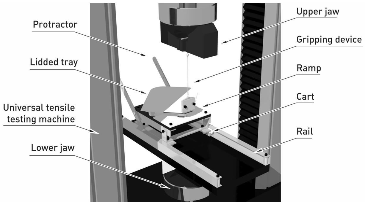
**Figure 4.5** – Variable angle test fixture.
