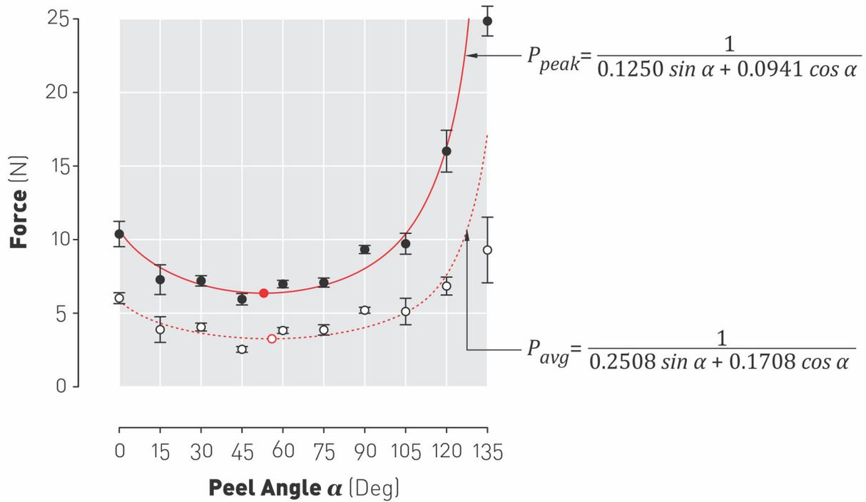
**Figure 4.11** – Condition A: Fitted curves over 0-135° range and experimental data for peak (●) and average (○) forces.
