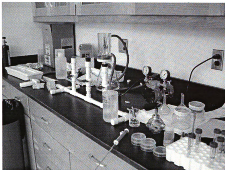
Figure C15: Membrane filtration lab set up.
