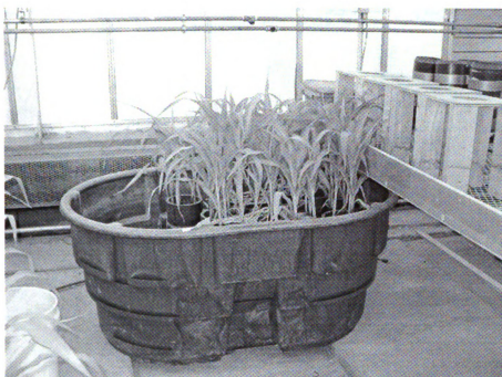
Figure C9: Saturation tank for saturated hydraulic conductivity.
