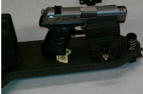
Figure 3.3: Ruger KP95DC 9mm pistol supported on firing stand for intact ammunition studies. For interpretation of the references to color in this and all other figures, the reader is referred to the electronic version of this thesis.
