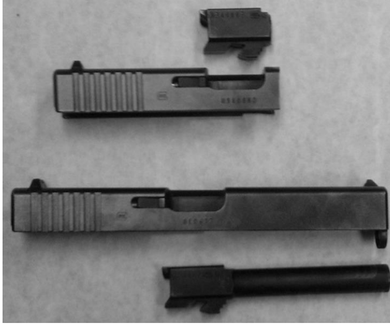
Figure 3.1: Glock 17 slide and barrel after removing barrel length (above) compared to unmodified components from another Glock 17 (below).
