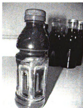
Figure 28. Picture of the PET bottle delaminating with tart cherry juice stored at room temperature (23°C, 50% Rh) after six months of storage.
