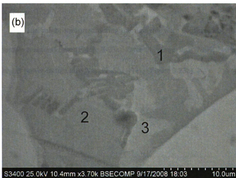
Figure 3-21. BSE images of sample from (a) bottom and (b) middle of the ingot \text{Na}_{0.5}\text{Pb}_8\text{Sb}_{0.5}\text{Te}_{10} .
