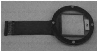
Figure 3.14: HiRA single-sided silicon strip-detector in a circular plastic container.
