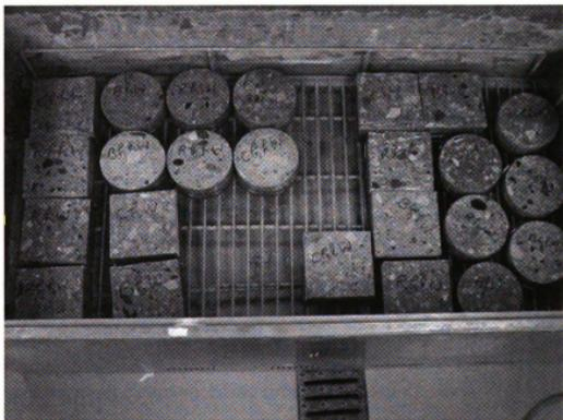
Figure 2. 13 1-D and 2-D sorption test specimens inside the test pan
