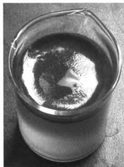
Figure 6.4: Adsorption of Manganese dioxide at the liquid-liquid interface – The nanosheets got adsorbed at the water-hexane interface to create a dry thin film with metallic shine from continuous evaporation of hexane
