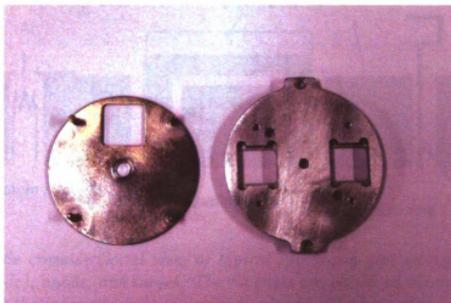
Figure 3.3: *This figure shows a typical substrate holder and a mask used in the Sputtering chamber. The substrate holder (shown on the right-hand-side) has two sample positions, only one sample is opened during the sputtering using the rotating mask (shown on the left-hand-side).*
