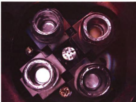
Figure 3.2: *The sputtering chamber showing six gun positions- four of them are large triode sources whereas the remaining two are small magnetron sources. In order to avoid the cross contamination, the plasma is confined using chimneys.*
