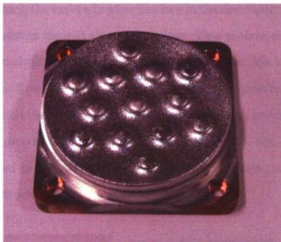
Figure 3.5: *The base target is made up of Palladium with Nickel plugs placed into the holes.*
