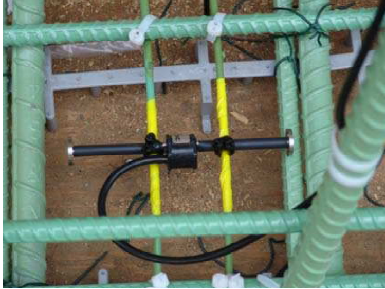
Figure 1.2: St. Anthony Falls Bridge: Structural deformations are measured by 195 vibrating wire strain gauges(VWSGs), 24 resistive strain gauges, and 12 fiber optic displacement sensors. (Fig source: http://buildipedia.com/operations/public-infrastructure/innovative-infrastructure-smart-bridges )
