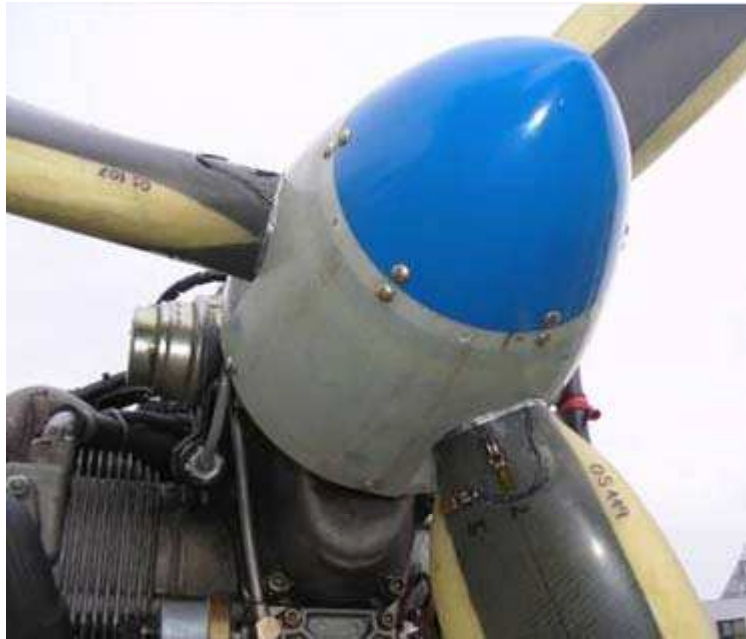
Figure 1.3: Fiber-composite propeller blades with LY41-6/350 strain gages from HBM, with tele-metric data transmission. (Fig Source: http://www.hbm.com/ )
