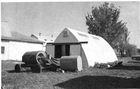
Fig. 1b. Supplemental heater used for drying shelled corn
