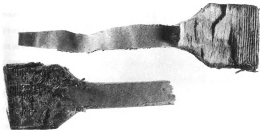
Figure 14.--Failure of a tangential bark specimen subjected to tensile loading.
