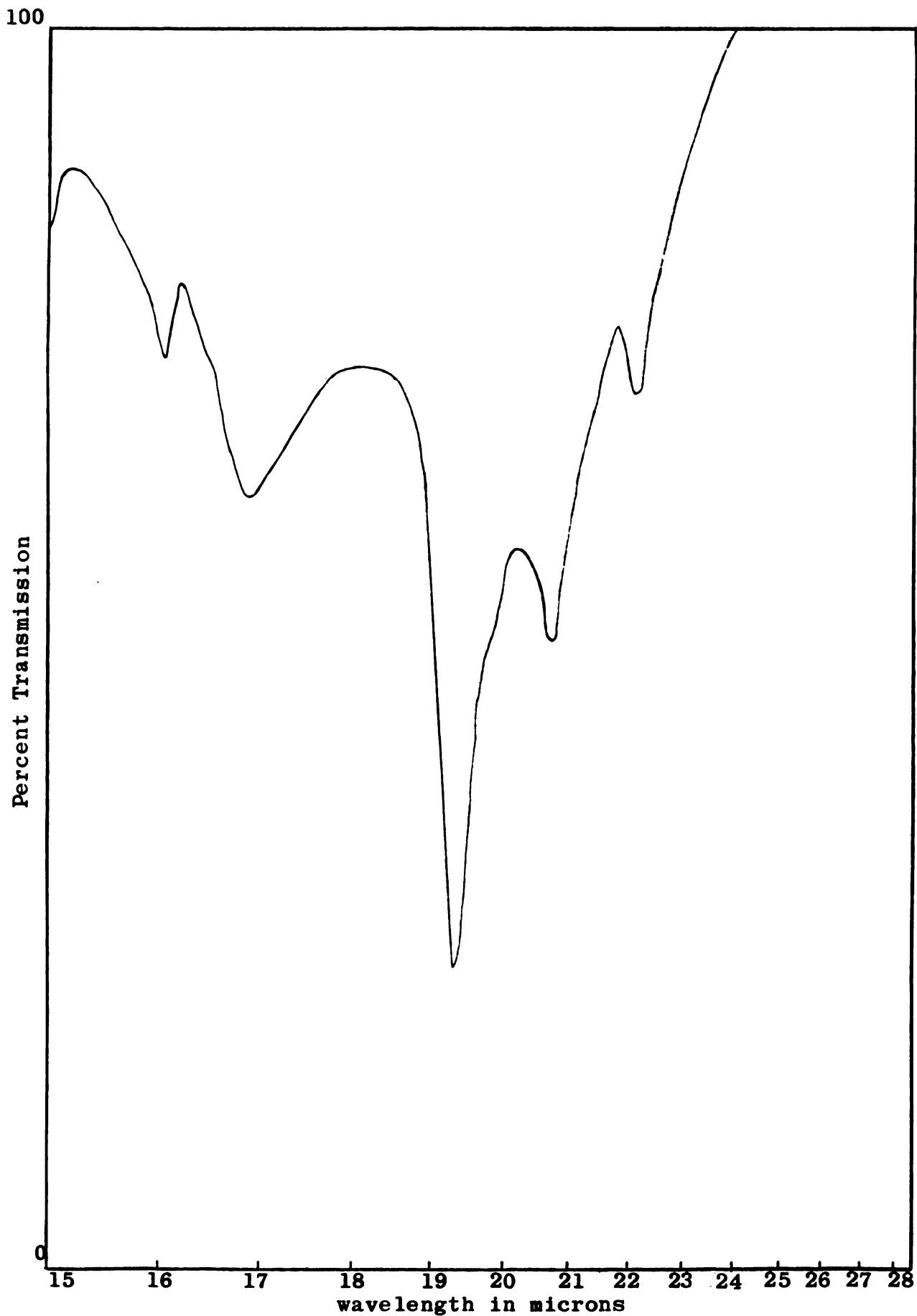
Figure 19. Infrared spectrum of cyclo-bis[tetraphenyldisiloxanylchromate(VI)] in the cesium iodide region.
