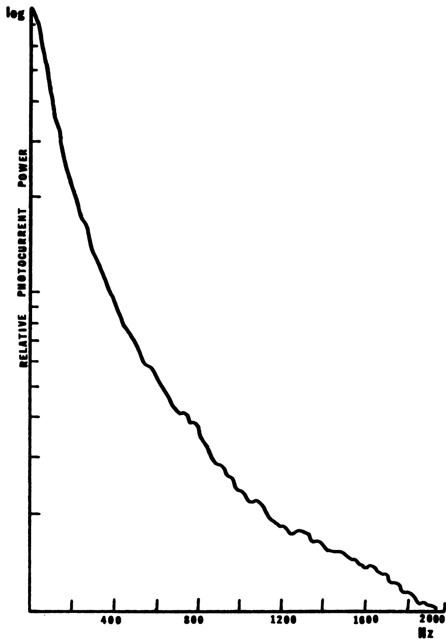
Figure 28. Photocurrent spectrum of light scattered from polystyrene latex at 35° scattering angle.
