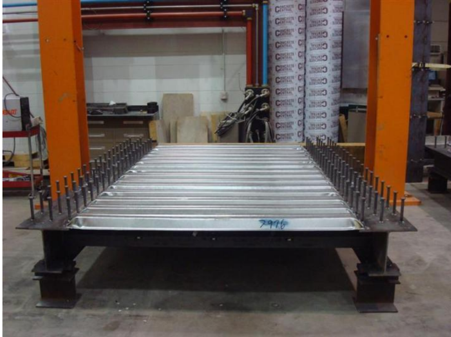
Figure 40. SIP forms front view
