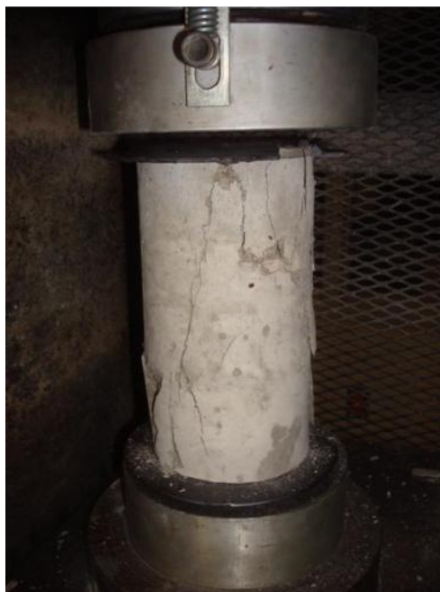
Figure 62. Concrete compressive strength testing
