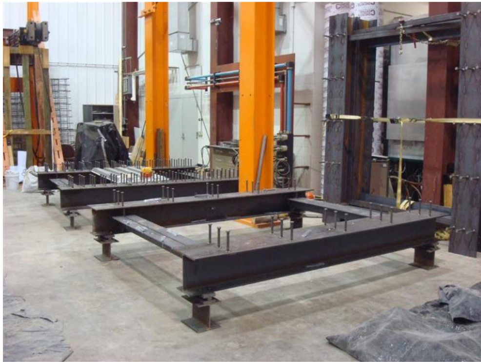
Figure 38. Test Unit Steel Frame Assemblies (Test units 1, 2, and 4)
