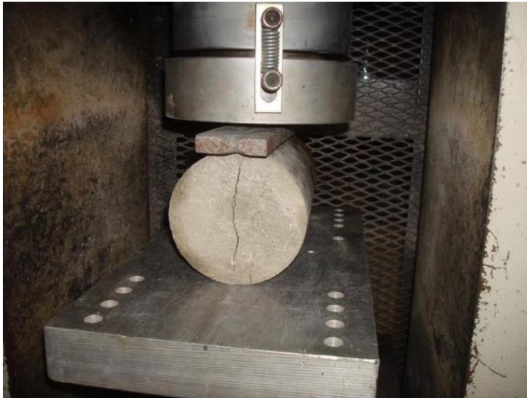
Figure 61. Concrete split tensile strength testing
