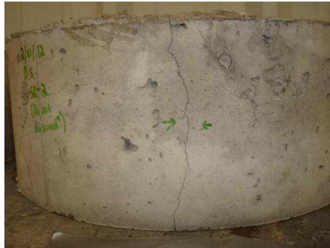
Figure 91. Ring test cracking (Ring 2)
