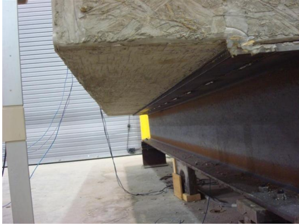
Figure 57. Completed test unit cantilever section (test unit 3)
