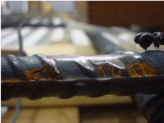
a) Ground and cleaned surface
