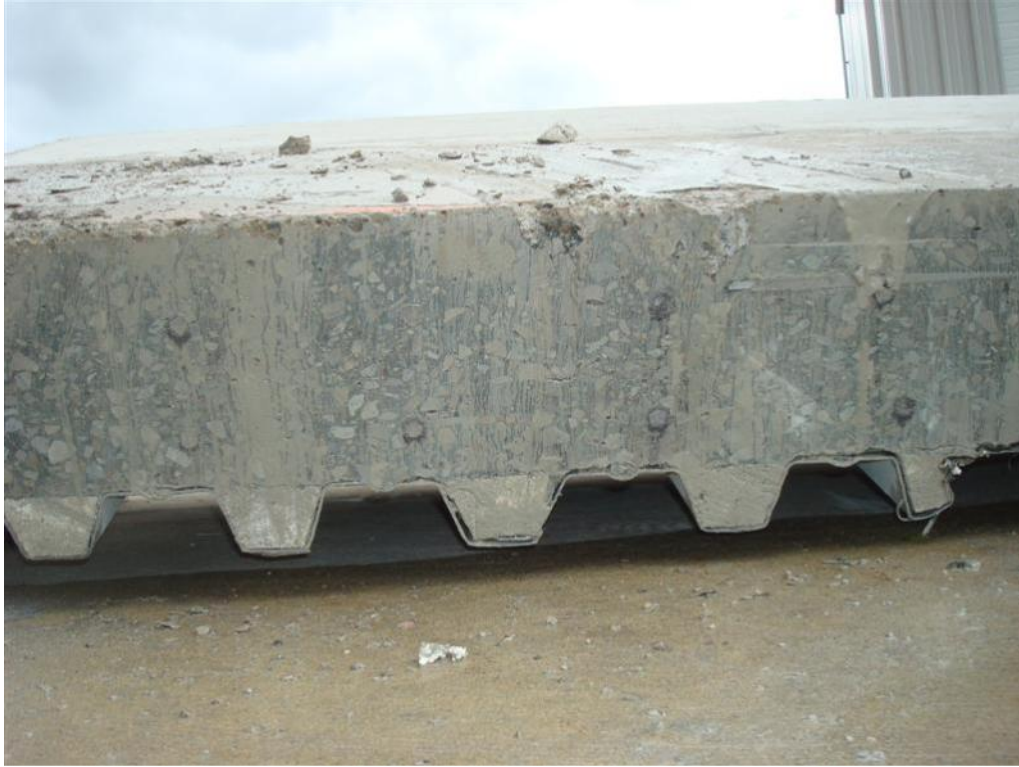
Figure 59. Test unit cross-section (test unit 4)
