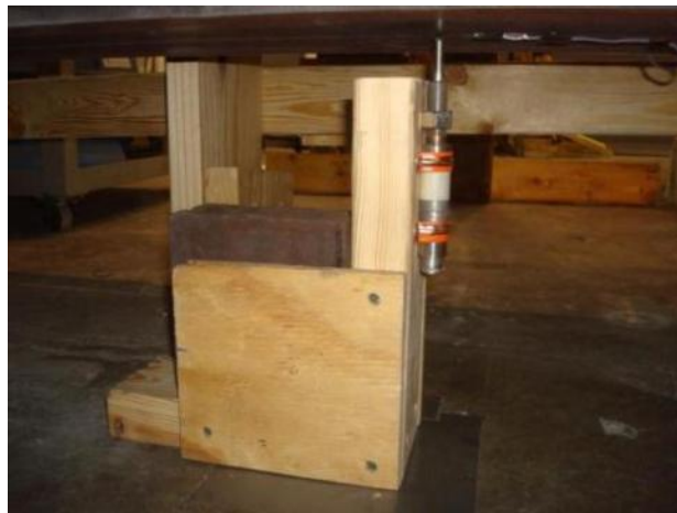
Figure 52. LVDT in place (mid-span of beam)
