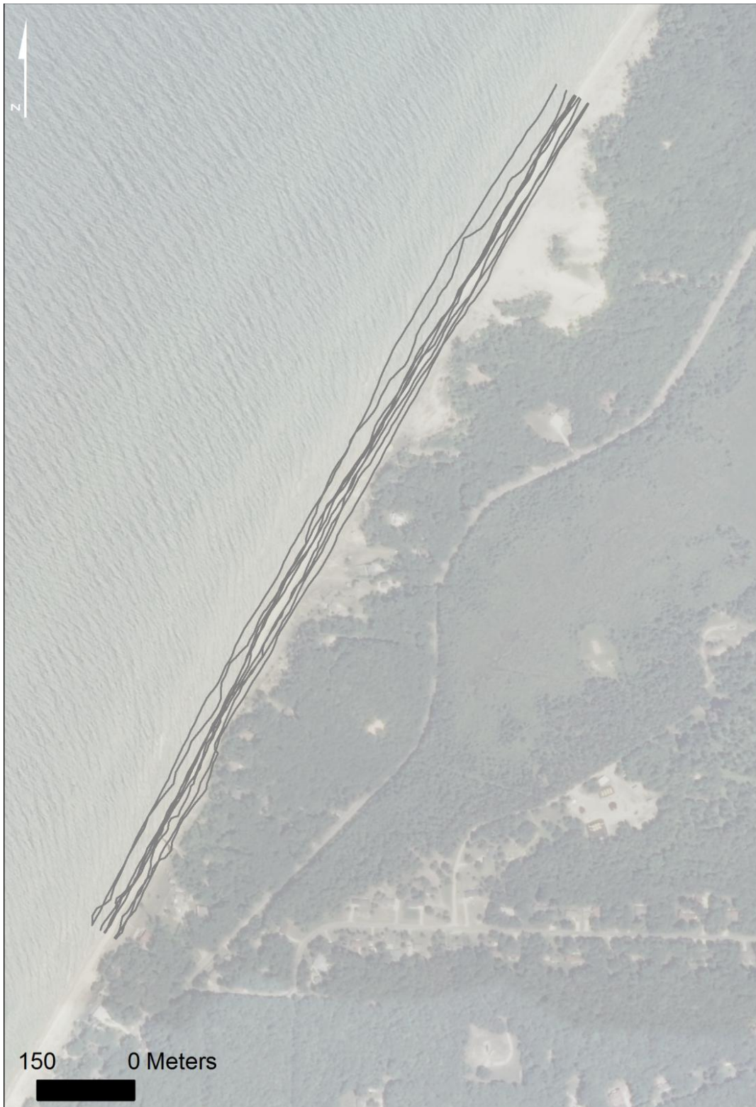
Figure 5.1: Variability in shoreline positions at the Manistee County site. Each gray line represents the shoreline position for one single year. The shoreline position fluctuated over a wide area.
