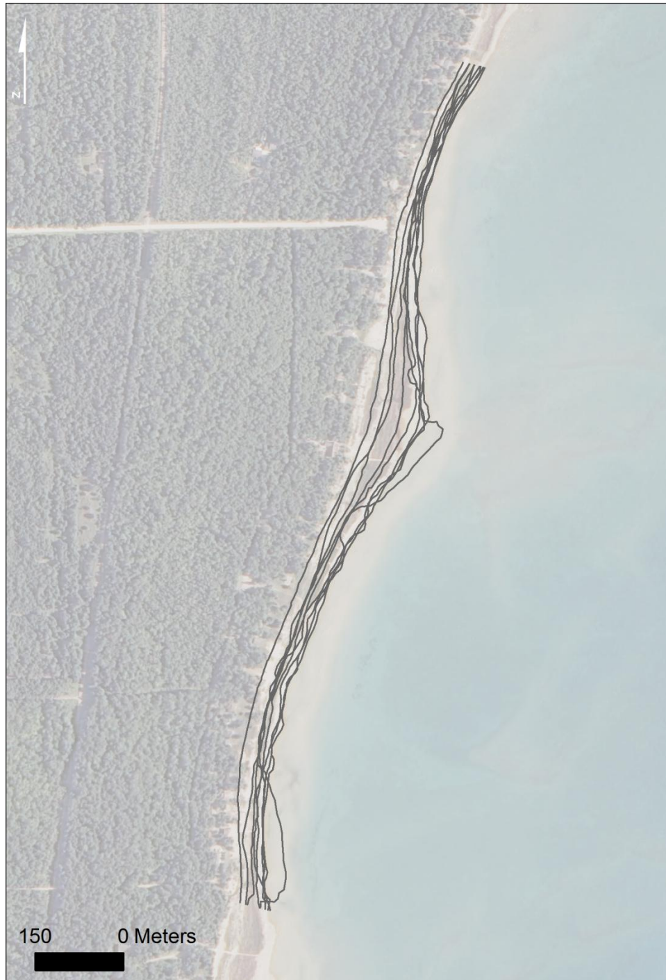
Figure 5.15: Variability in shoreline position at the Alcona County site. Each gray line represents the shoreline position for one single year. The shoreline position fluctuated over a wide area.
