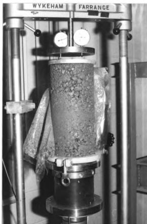
Figure 6.17. The honeycomb structure of Sample 31 for an extremely low mortar content.
