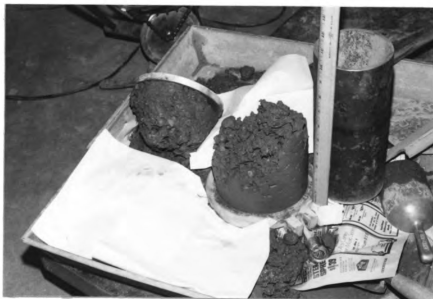
Figure 6.6. Two examples showing the dead zone of failed samples.
