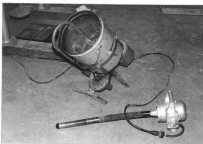
Figure 4.3. Mixer and vibrator.
