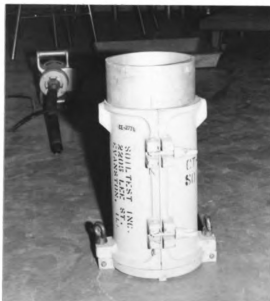
Figure 4.4. 6 in. x 12 in. mold with a 2 in. extension tube on top.
