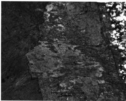
Figure 3a: Perthitic alkali feldspar in felsite Marl4A.
