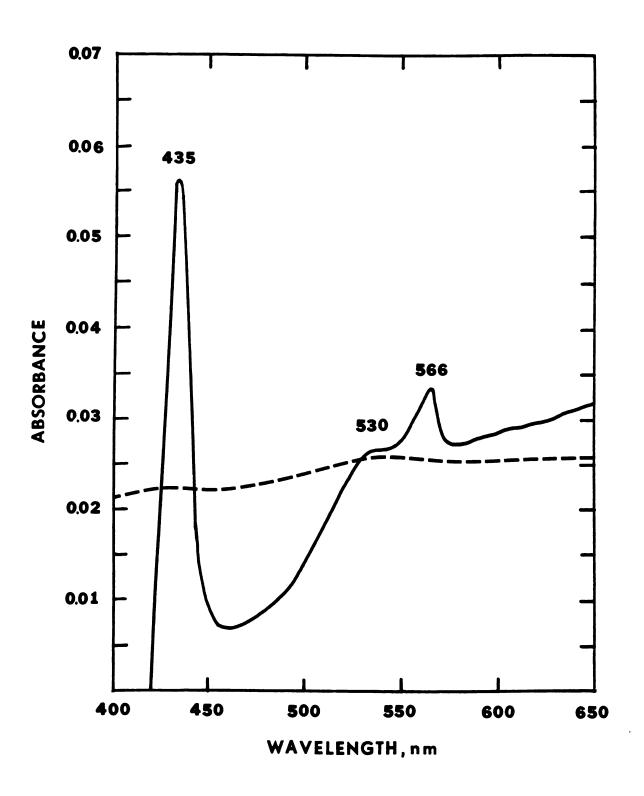
Figure 16.--Difference spectra of a protoheme extract (10.8 mg of protein per ml pyridine-KOH) of <u>C. bovis</u>. Airoxidized versus air-oxidized (broken line) and dithionite-reduced versus air-oxidized (solid line) difference spectra. Other experimental conditions were as described for Figure 8.
