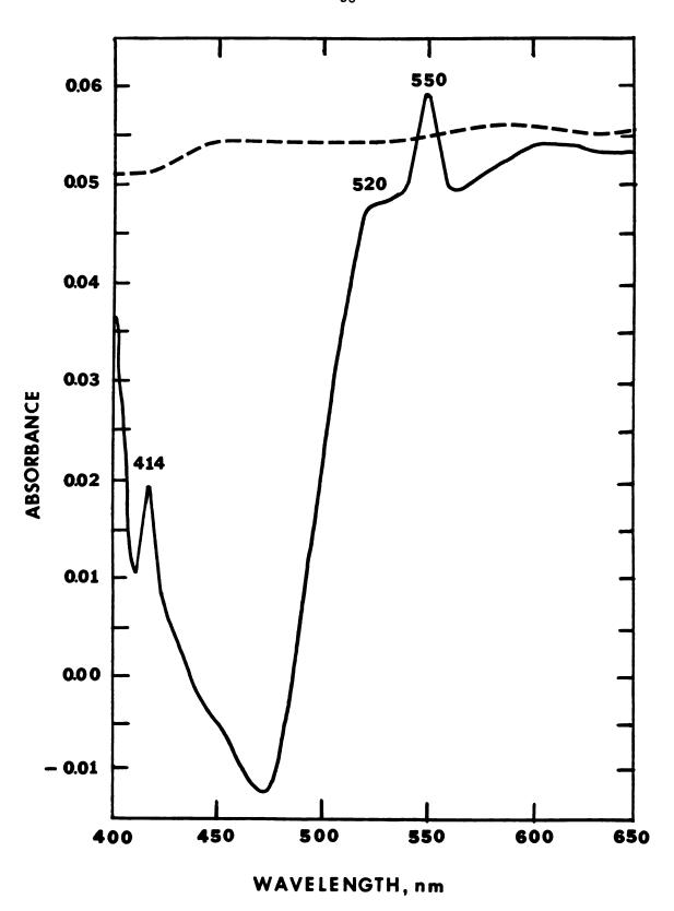
Figure 13.--Difference spectra of a cell extract (12.3 mg of protein per ml) of  $\underline{C}$ . renale. Air-oxidized versus air-oxidized (broken line) and dithionite-reduced versus air-oxidized (solid line) difference spectra. Other experimental conditions were as described for Figure 8.
