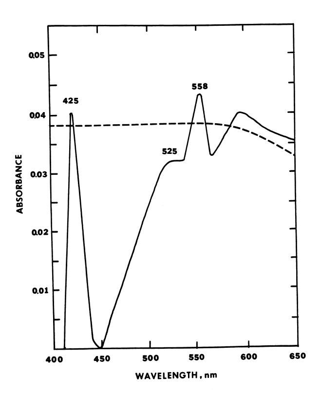
Figure 22B.--Difference spectra of a protoheme extract (7.2 mg of protein per ml pyridine-KOH) of <u>C</u>. <u>diphtheriae</u> 2. Air-oxidized versus air-oxidized (broken line) and dithionite-reduced versus air-oxidized (solid line) difference spectra. Other experimental conditions were as described for Figure 8.
