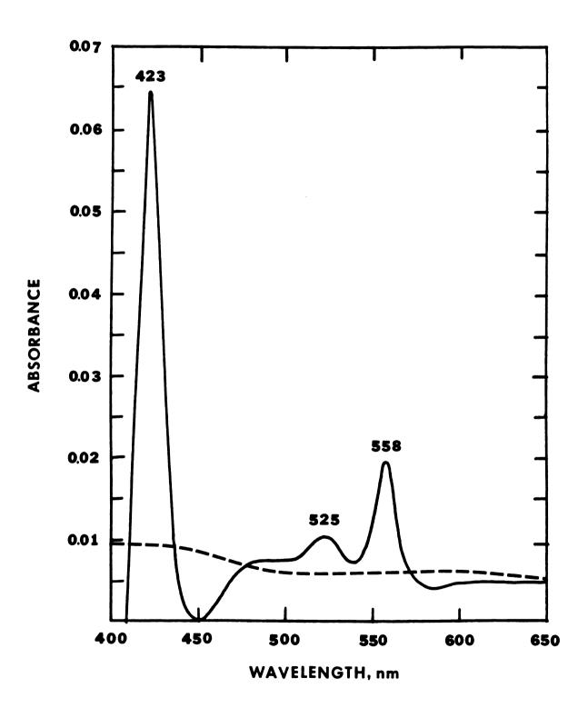
Figure 10.--Difference spectra of a cell extract (10.9 mg of protein per ml) of <u>C</u>. <u>equi</u>. Air-oxidized versus air-oxidized (broken line) and dithionite-reduced versus air-oxidized (solid line) difference spectra. Other experimental conditions were as described for Figure 8.
