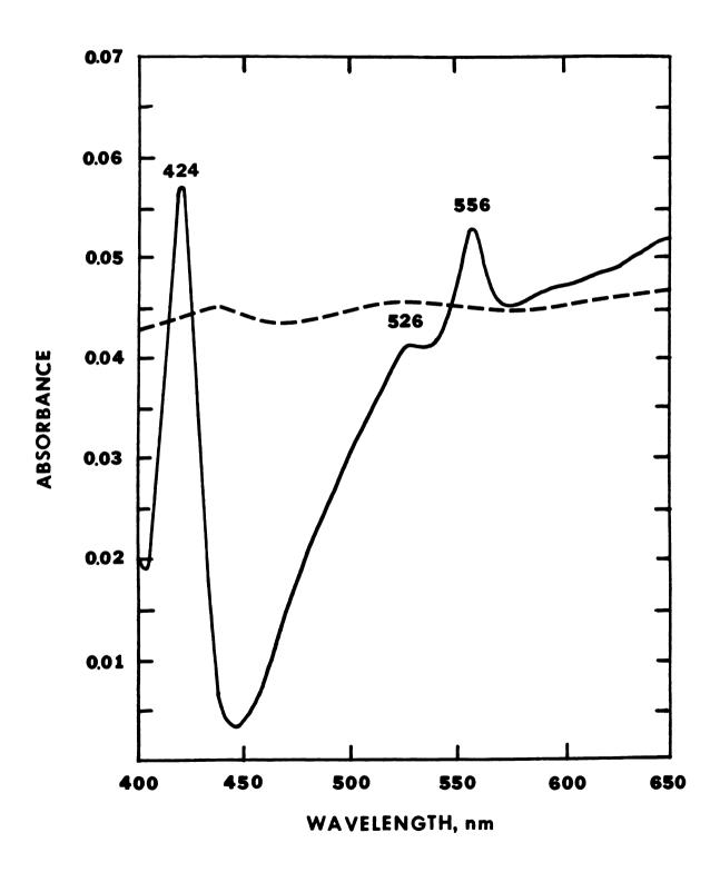
Figure 19.--Difference spectra of a cell extract (7.7 mg of protein per ml) of <u>C. pseudotuberculosis</u>. Airoxidized versus air-oxidized (broken line) and dithionite-reduced versus air-oxidized (solid line) difference spectra. Other experimental conditions were as described for Figure 8.
