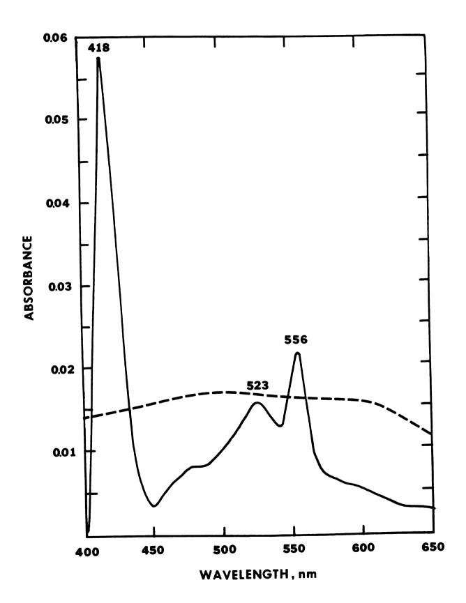
Figure 21A.--Difference spectra of a cell extract (5.9 mg of protein per ml) of <u>C. diphtheriae</u> 1. Air-oxidized versus air-oxidized (broken line) and dithionite-reduced versus air-oxidized (solid line) difference spectra. Other experimental conditions were as described for Figure 8.
