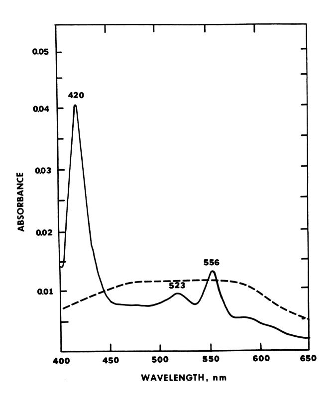
Figure 22A.--Difference spectra of a protoheme extract (10.9 mg of protein per ml pyridine-KOH) of <u>C</u>. <u>diphtheriae</u> 1. Air-oxidized versus air-oxidized (broken line) and dithionite-reduced versus air-oxidized (solid line) difference spectra. Other experimental conditions were as described for Figure 8.
