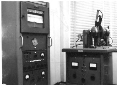
Figure 2. "Norelco" x-ray diffraction unit with recorder.
