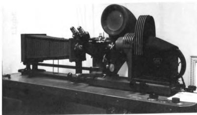
Figure 3. Balphot Metallograph with camera attachment.
