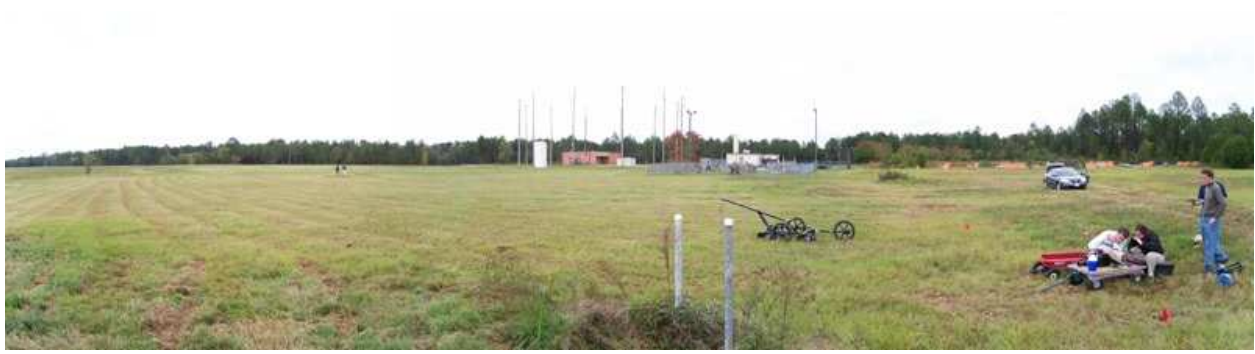
Figure 1.5 Panoramic view of the site showing the source location (metal pipes in the center-front) and GPR data collection setup (on the right) (photo courtesy: Kaya Diker).
